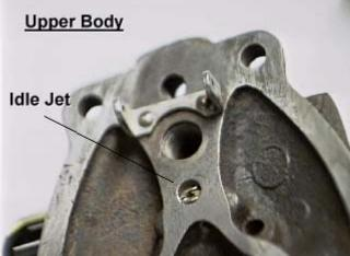
Next to the float seat is the idle jet seat. This is the jet into which the idle screw/needle fits when the carburetor is running on your tractor. Removing this tiny jet is also tricky since its bearing surface is even smaller than the float seat. Use the widest straightslot screwdriver that will fit the casting hole and fit into the idle jet slot. Same as before, keep the screwdrive from slipping and the jet will come out.
