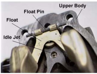
A steel pin holds the float in the upper body. Slide the pin out of its ears to release the float. Shake the float and listen for any liquid inside the floats. If there is liquid inside either float, replace the float and set in a safe place.
