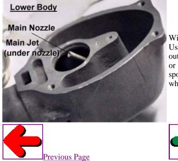
With the venturi out, remove the Main Nozzle. Use a nutdriver or deep socket to get the nozzle out. Make sure that you don't cock the nutdriver or socket to one side or you will bend the nozzle spout which will keep it from breathing properly when reassembled.
