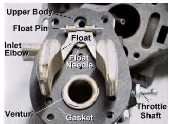
Check the float level by holding the upper body with its manifold studs down so that the float tang rests on the float inlet needle and measuring the distance from the gasket to the closest part of the float. Adjust the tang by bending to get 1/4" clearance.
