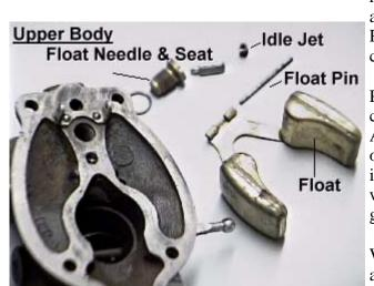
Drop the upper carburetor body, idle jet (seat), the power mixyure screw/spring and idle mixture screw/spring into the parts basket and lower it into the cleaner. Make sure it is completely covered. Watch out for splashes!
