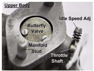
Note the stampings on the butterfly valve so that you can reinstall it exactly as it came out of the throttle body. Make sure that the rebuilt kit has replacement screws, and throw the old ones away.
