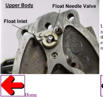
Underneath the float and held in by the float tang is the float needle. Pull it out and compare it to the new one in the rebuild kit. The needle will either be made entirely of steel or will have a rubber tip. Either version will work fine.
