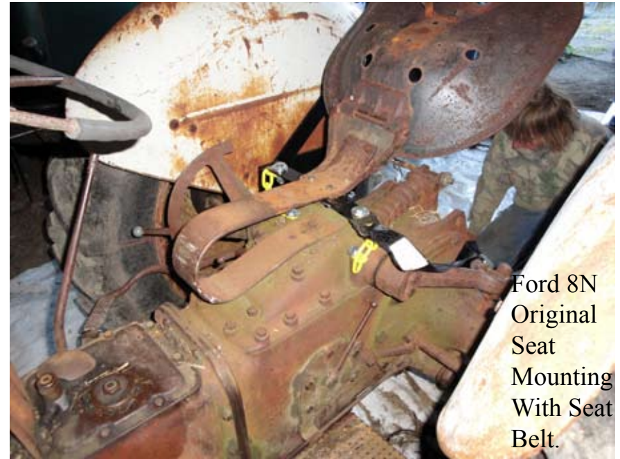
Ford 8N Original Seat Mounting With Seat Belt.
