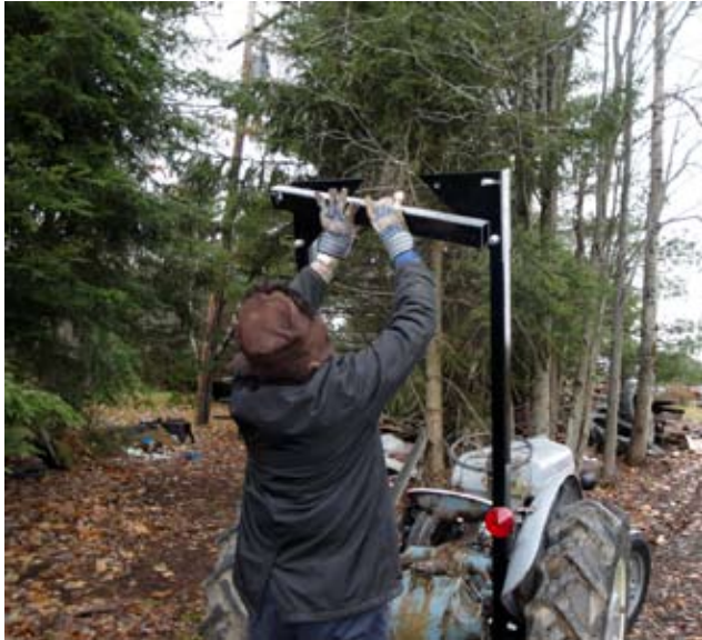
Steps 17 -19 Installing Cross Bar Rear View
