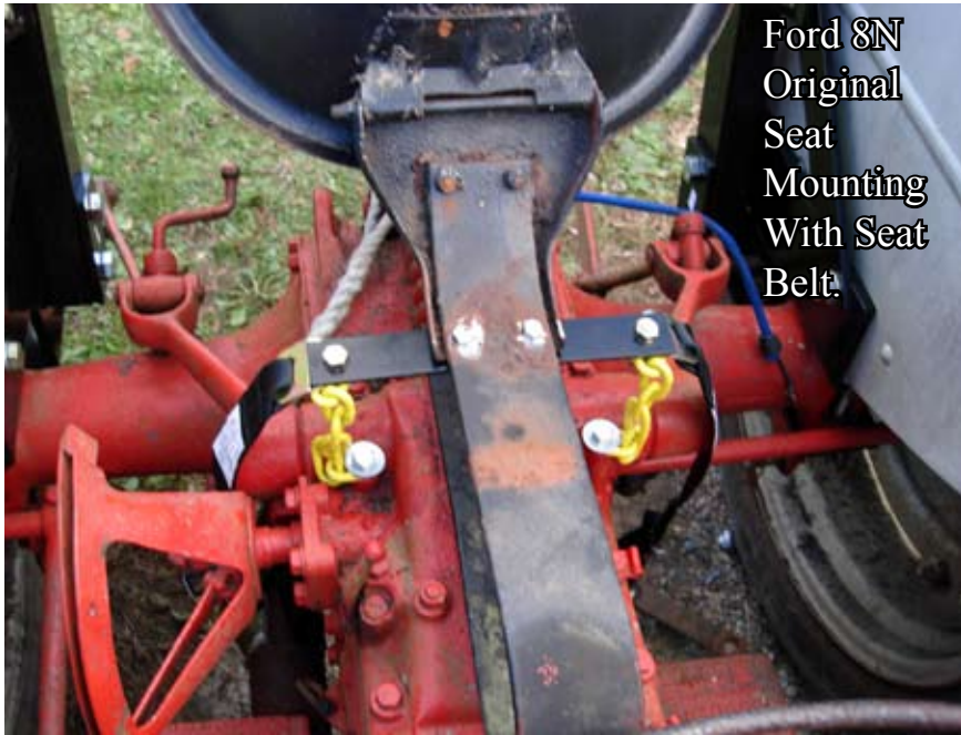
Ford 8N Original Seat Mounting With Seat Belt.
