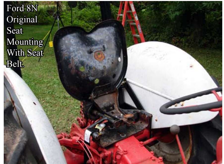
Ford 8N Original Seat Mounting With Seat Belt.
