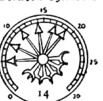
Leaky Head Gasket Between Cylinders
