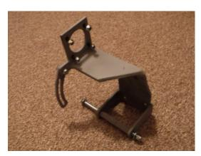
This is a prototype bracket designed to mount a hydraulic pump to the 8N side-distributor block, without having to stack two mounts on the studs. This bracket replaces the original generator bracket. This particular one is for an alternator. The generator uses the original adjuster behind the water pump.
