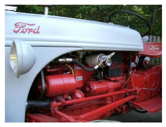
This photo shows most of my system, with optional accessories. I added a suction line strainer with a gauge, so I can see when it's time for a new strainer. The gauge was not needed. The pump starts to cry with any backpressure increase as the strainer gets clogged. This system needs a dual strainer to reduce restriction in the suction line.
