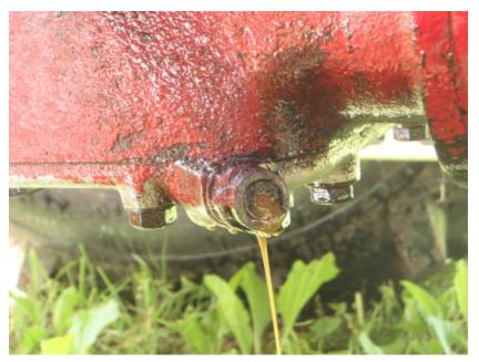
This is what happens if you use unrated pot-metal fittings from Lowes. The fitting I originally used was a simple street elbow threaded into the original test port plug. It lasted until something hit it and snapped it off. 2 GPM is a lot when the hot oil is spraying everywhere, and filling your shoe. Use rated hydraulic fittings.
