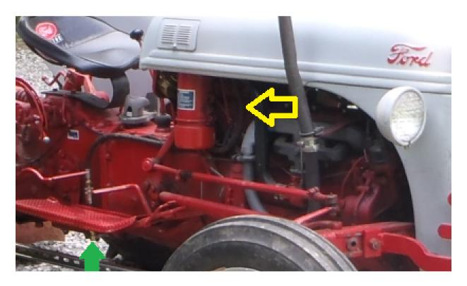
This photo shows the route I used for the High Pressure Hose. The yellow arrow is where the hose appears, runs along the top of the transmission with the tail light wires, and then drops to the test port under the footboard. The green arrow is pointing at the test port.
