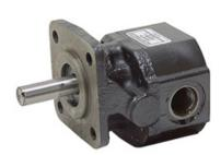
I am using a BARNES Model# 1003044 SAE 8 CW 0.194 cu in displ, 3000 PSI, 4000 RPM max, 3 GPM @ 3600 RPM, CW rotation, Mount 4F17, Shaft 1/2" dia x 1-1/2", IN and OUT Ports = SAE 8 (3/4-16),
