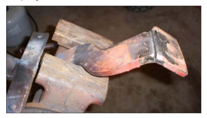
Here's the finished bumper prior to painting. The ends can be fine tuned at this point to make sure they all line up.
