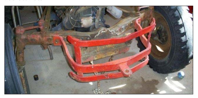
From this view we can see that even the upright pieces are bent. Considering the number of bent parts I think it's best to disassemble the bumper, straighten out each part, and re-assemble.
