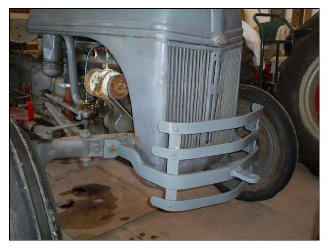
This is my bumper as I received it. The top bar is bent, the 2nd one down is missing, the bottom bar is bent, and the main bar is sprung so the bumper is too wide to line up with the axle bolt holes.
