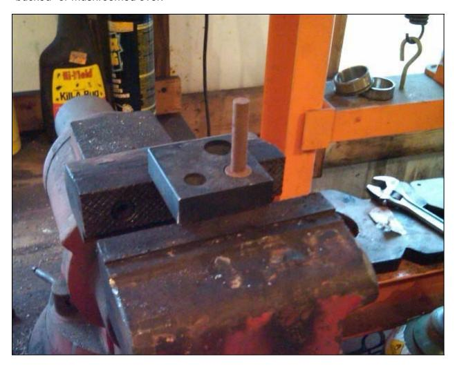
The next piece is used for bucking the rivets (mushrooming over). These tools are sometimes found in old hardware stores or you can make one like I did. Use a chisel as they are high carbon steel which makes for a better tool. I cut the end off the chisel and drilled a 1/2" hole in the end. I later shaped it a little using small Dremel stones on a Dremel tool. My tool does not produce an exact round rivet head but its closer than just using a hammer.
