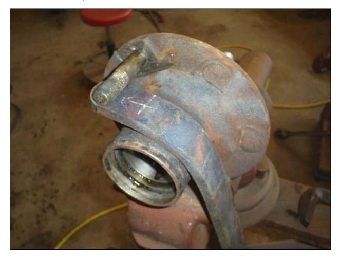
This bending requires some skill as you heat a small area and bend, move a little and repeat. While time consuming it's obvious what can be produced. Start by getting the center bent correctly the move on to one side and keep checking. The difference between an ok job and an excellent one is the patience to keep re-working the part until its right. None of these parts were produced right the first time. Once the center and the corners fit I marked and trimmed the ends to match the existing bars.
