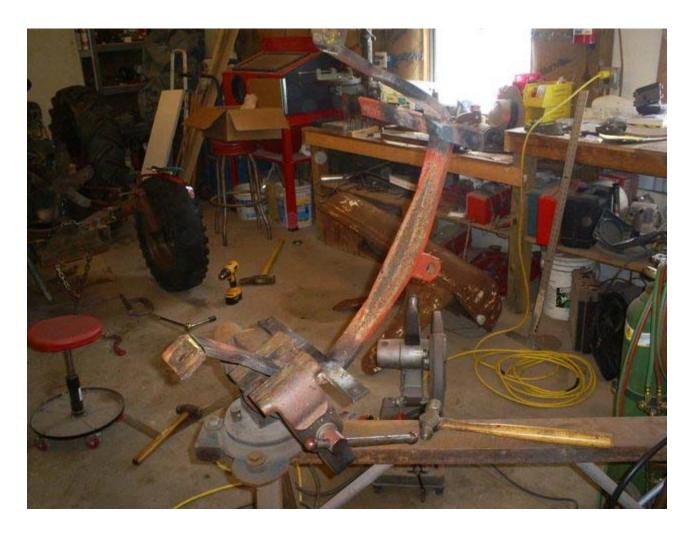
I also did not like the way the bolt tabs matched up to the front axle. I used an abrasive cutoff wheel mounted in an air tool and cut a slit in the mounting tabs then bent them until they matched the front axle. Once adjusted, I welded them back up and dressed them up with grinders.
