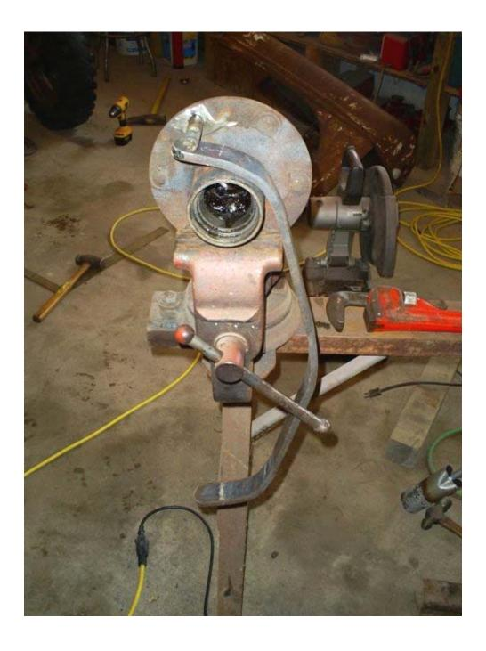
Once the bars were properly bent I tacked welded them on from the back and drilled the existing rivet holes through. Care needs to be taken to ensure the new bars are centered over the old holes. Once the holes were drilled I knocked the bars back off and cleaned up the tack welded areas.
