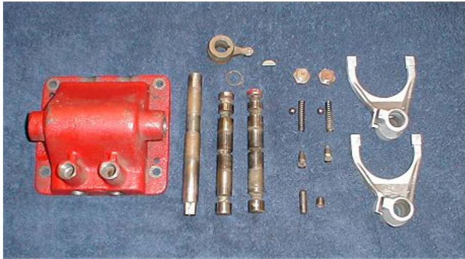
The disassembled top cover and all the parts.
