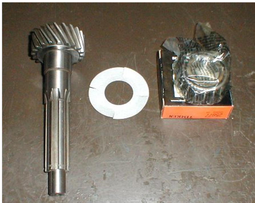
The new output shaft, slinger and bearing ready to assemble.
