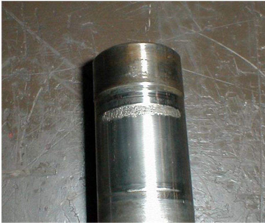
An example of galling on the rear end of a countershaft bearing diameter. More junk.
