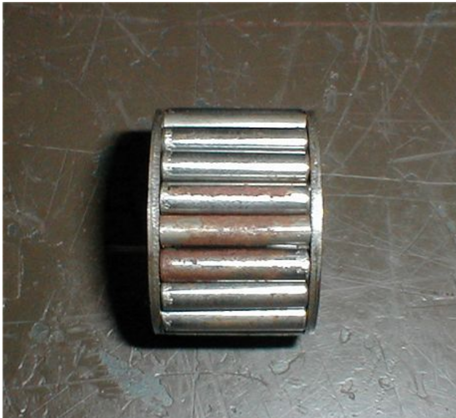
This needle bearing has rust and pitting on the rollers. The rollers are also starting to crumble on the left end. It's very rare to find any of these that are good enough to use over again. Replace 'em.
