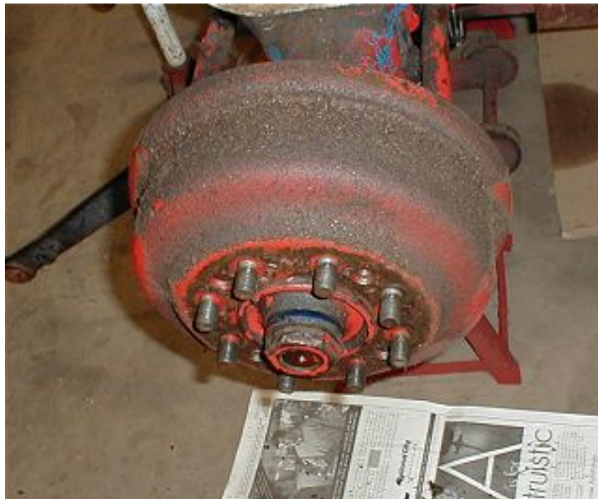
A common sight, the oil soaked rear brake drum on an 8N
