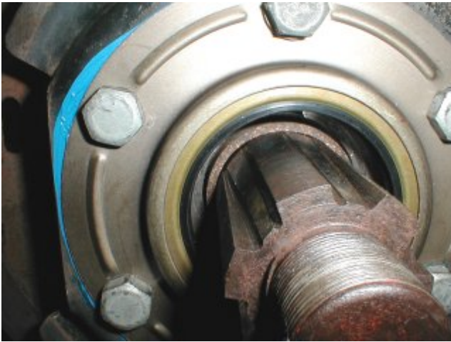
8N 4284 axle to hub cork seal installed
