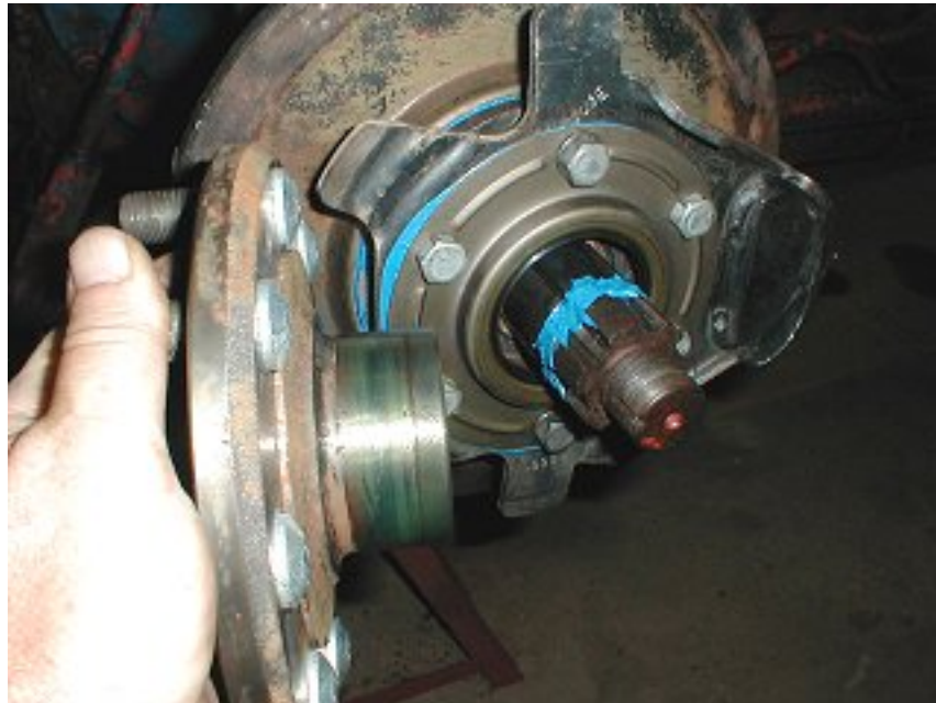
Installing the hub
