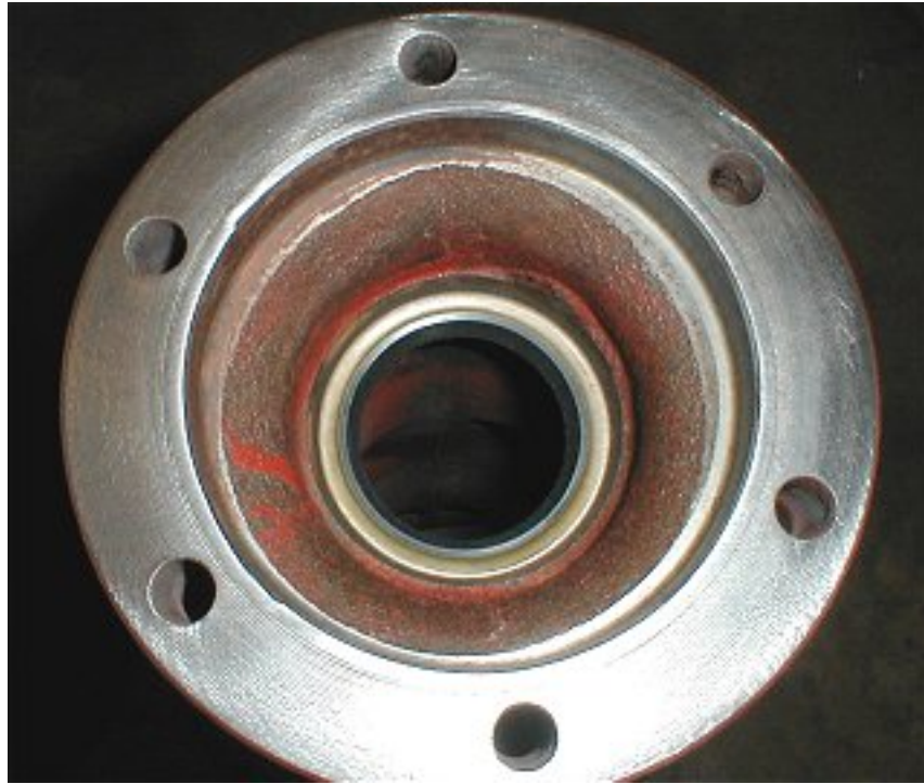
The inner seal on the '50 - '52 models
