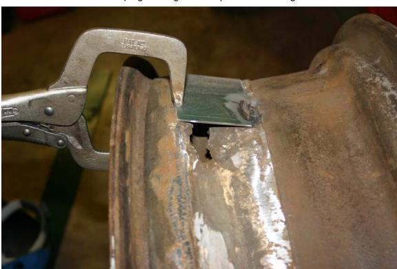
Joining the segments end to end:
