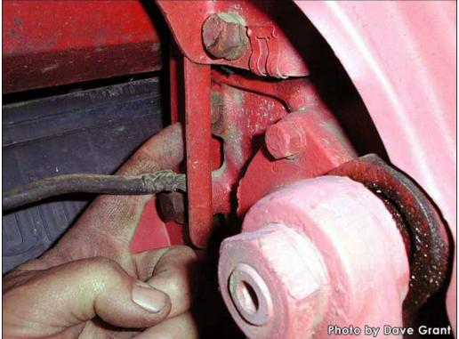
On April 20, 1951, the first oil filler plug was discontinued. The hole is filled with metal, completely sealing it. At this time the cap screw on the right hand side, which secures the instrument panel support to the steering housing, was used as the filler plug.
