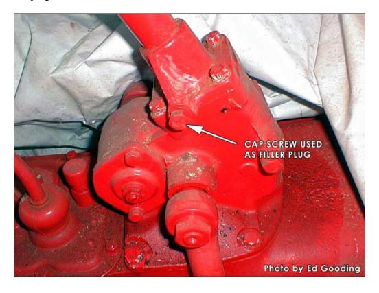
The housing should always be filled to the level of the cap screw hole to insure that the top bearing (8N-3571), receives lubrication. Fill when the level falls below the cap screw.
