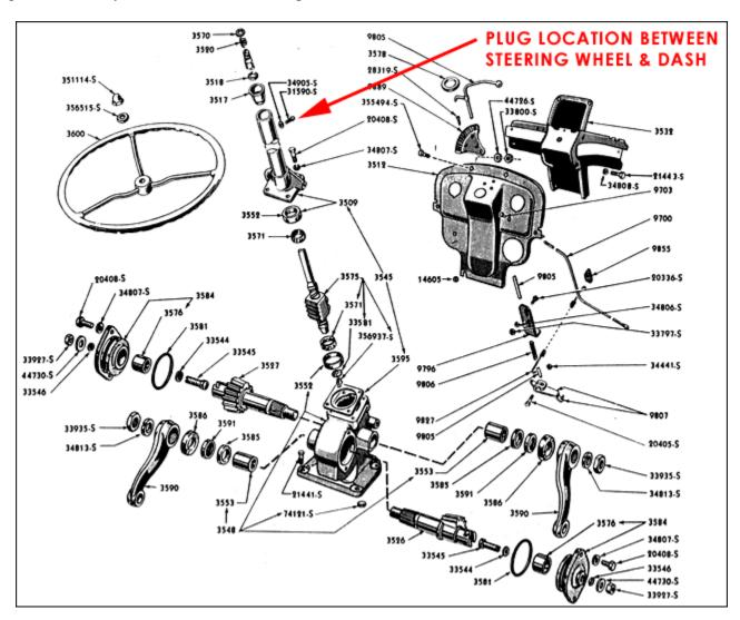
The plug used was a 1/4"-28 x 5/6" fillister head screw. This was a handy to get to location and when filling added oil to the upper steering thrust bearing.
