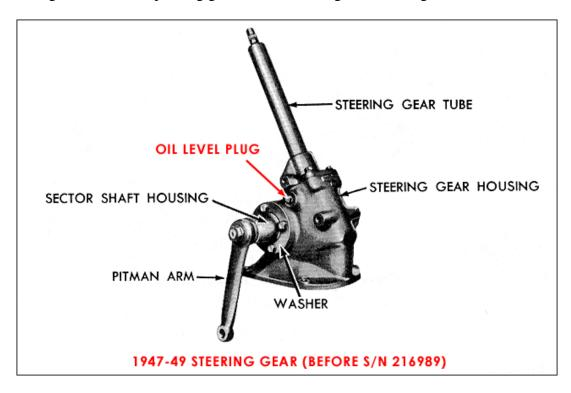
In September 2, 1949, the 8N-3503 steering gearbox assembly was replaced with a new beefier steering gearbox 8N-3503-B starting with serial number 216989.
