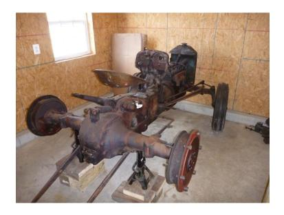
The rear axles and trumpets were pulled and replaced with smooth axles. Once accessed, we found that the inside of the axle housings, hydraulic pump, and transmission were caked with "mud" from old fluids and simply from sitting for so long. I'm sure the barn fire didn't help this any.
