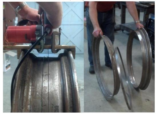
Once the Rim was cut into two pieces, I got to work on clamping it down to my welding table and tig welding it back together, while my father started removing the loops from the old rim.
