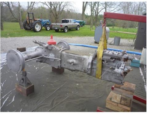
After a quick hand sanding and cleaning of all the sand off the tractor, a first coat of self-etching primer was applied to prevent it from rusting.
