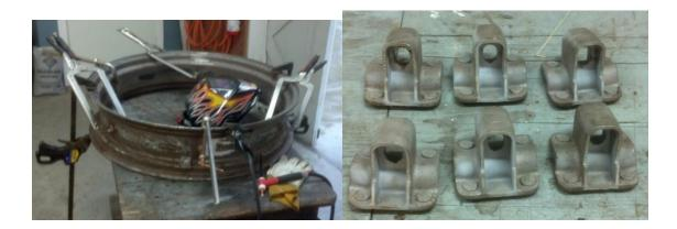
Using the original wheel center and bolting the loops on to it, we got the loops in the proper spot on the rim. We then marked their hole locations and drilled holes in the rim. Then, welding on the loops from the inside gave it the appearance that they were riveted on like the originals.
