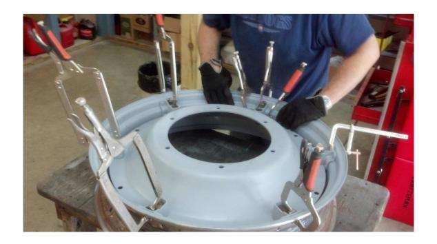
Hours of grinding, sanding, priming, and painting later the rim was complete and ready to be used again. Since the original rim was removed prior to the barn fire of 2009, the original bolts and nuts for the loop rim were lost. Finding ones that have a 1-1/16" head with a 5/8-24 thread (not a standard size) was not an easy task. So, to the lathe I went and made identical nuts and bolts out of 1-1/4" hexagonal bar stock.
