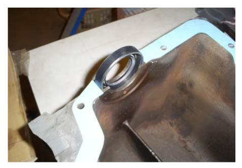
The next step is to confirm that the oil pickup tube lines up with the oil drain hole. The pan is placed into position and confirms that the oil plug will install without interference. If there was a problem you can remove the pan and gently align the pickup tube. The pan was painted as part of a test of different paint products and has no significance in the assembly. Once happy set the pan aside.
