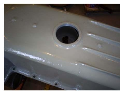
Install the camshaft. Lube the 3 journals where the shaft runs as well as the areas on the camshaft where it runs in the block. Ensure that the timing marks line up. This cam gear is stamped .005 which indicates its oversize for thrust wear.
