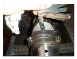
Once the crank is in slip the front pulley and nut on and see that the crank will turn. It may be tight initially but will loosen up. Make sure the rear seal ends do not get lube on them. On my motor, the crank with the main bearings installed and top half of the rear rope seal required around 10 ft/lbs to torque to rotate. The initial rotate is a little higher and quickly lessens as the crank is spun. It should rotate freely with no tight spots or binding.
