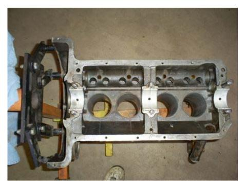
Carefully set the crankshaft in place. Cut a strip of Pastigague (.001-.003) the width of the each main bearing journal and lay on the crankshaft journals. Place the other bearing shells in the main caps and install in place with the arrows pointing towards the front of the block. Torque the bolts/nuts to the correct setting.
