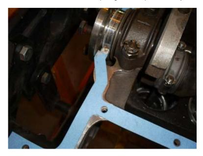
This is the front seal with the pan gasket in place, ready for sealer and the oil pan installation.
