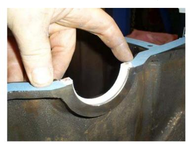
Prepare the front seal on the pan. Place the 1 piece neoprene seal in its groove and cut the pan gasket so that it butts up against the seal.
