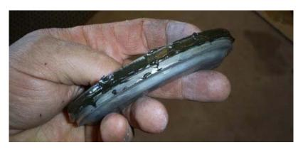
Prepare for rear seal installation. With the rear seal retainer in place set the pan gaskets on the block lining up with all the holes. Press on the ends where the gaskets overlap the rear seal groove leaving an indentation in the gasket. These marks will be used later for trimming.
