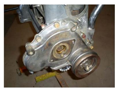
Oil Pan installation. The rear seal was installed earlier. For the rear seal we are not overlapping the seal with the pan gasket so the rope seal is cut flush to slightly higher than the block, and slightly taller than the pan and gasket creating a slight interference. Lube the face of the rear seal with assembly lube keeping the ends clean.
