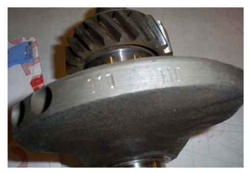
Verify that your bearings match the crankshaft. This bearing shows .010 meaning .010 undersize. It's nice to see it on the box but check the bearing.
