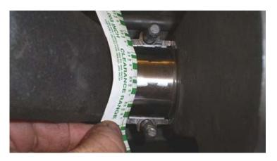
As each piston is installed, check the rod side clearance the same way you checked the crankshaft end play. Gently tap each rod to 1 side then check the clearance between the cap and crankshaft.
