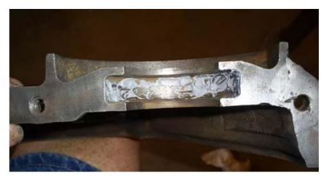
Once on your motor should look like this. Use a temporary bolt for the lower governor bolt hole to hold the parts in place as the sealant dries. Gradually tighten up all bolts that contain the timing cover and governor mounting plate.
