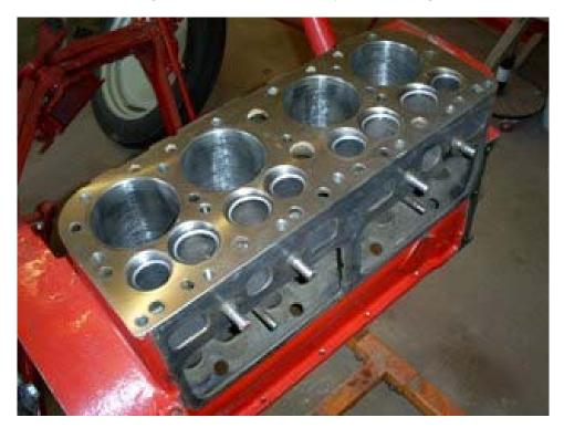
With the valves lapped it's time to do a final cleaning of the block and crankshaft. Pick up a set of brushes at the hardware store. These came from Harbor Freight and cost less than \$10.00 for the set.
