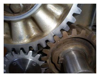
Check the gear lash on the crankshaft and cam gears. Here I've cut a feeler gauge to fit between the teeth. If the gap exceeds the tolerance a new cam gear is probably in order.
