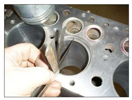
Assemble the pistons. Install the wrist pin keeper in one end, then slip the wrist pin in and the keeper from the other end. Use engine assembly lube on the pin and inside of the rod bushing. There should be virtually no play with the pin in the rod and should only move where intended. Side to slide movement is normal. Ensure that the keepers are seated properly in the pistons. If the keeper comes out the wrist pins will work loose and hammer the cylinder sleeve forcing a rebuild.
