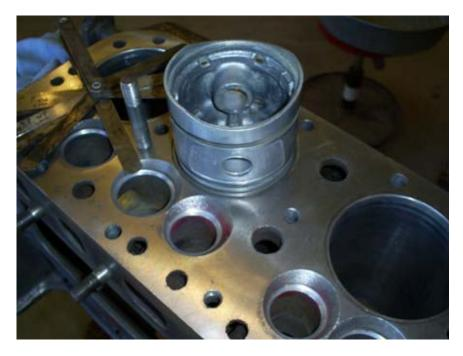
Measure the gap in the end of the ring and verify its correct. The rings are fragile so handle with care. All the ones I've checked were on the large end of acceptable out of the box but this is the only reliable way to know they are correct.
