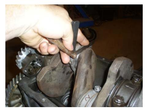
Rotate the crank following the installation of each piston. While new pistons/rings/sleeves will have some drag the crank should still rotate smoothly. On my motor with 2 pistons installed the torque required to turn the crank was around 20 ft/lbs.
