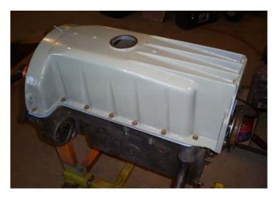
Congratulations on the main engine block assembly. In part 3 we will begin with the valve train installation and continue the assembly. Allow the gasket sealer some time to cure before rotating the crankshaft
