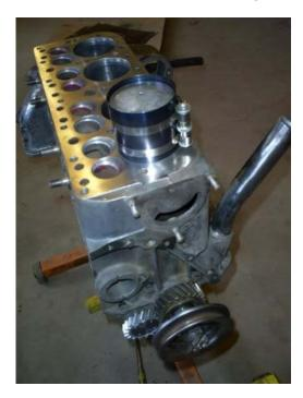
With the connecting rod in, place a strip of Pastigague on the crankpin and install the bearing shell and cap and torque to specification. Remove the cap and confirm that the rod bearing clearance is correct. This is the only reliable way to know that the clearances are correct. Once happy, clean the Pastigague off, lube the other bearing shell and install the cap. Repeat the process for the remaining pistons
