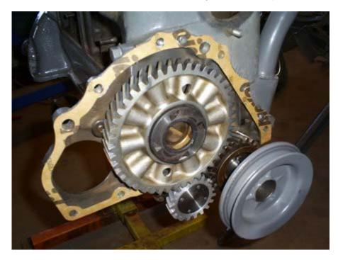
Add some sealant to the grove that holds the front crankshaft seal. With the seal spaced out from the motor, carefully lower the front cover onto the seal then work the cover back onto the motor lining up on the 2 dowel pins. Once located gently work the pulley back towards to motor. Install the crankshaft nut and tighten.
