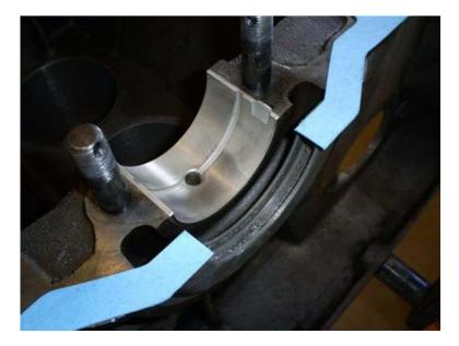
With the retainer in place, work the rope seal into its groove. Use a large socket and work it in which is easier with a dry gasket (wet gaskets swell). Once in, trim the ends flush to just slightly higher than the block. Use a sharp knife producing a clean cut. With the seal in place carefully apply engine assembly lube to the crank side of the rear seal keeping it off the ends of the rope. Repeat the lube application after the seal has set for a while
