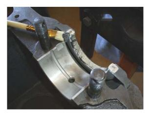
Using engine assembly lube, lube all the bearing shells including the sides of the center bearing, this is the crankshaft thrust bearing. Place the crank back in the block and install the main bearing caps, note the center and rear cap have arrows pointing towards the front.
