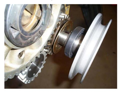
The governor plate and gasket are installed with sealant. Pay attention to mating lines keeping them flush and don't fully tighten the screws yet. Note that the camshaft thrust washer has been added.
