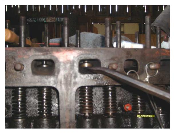
Place the pry bar on top of the valve guide.
