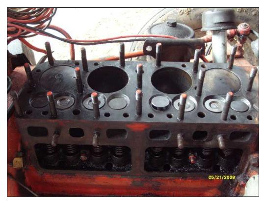
**Step Two:** Get the old parts out. One valve was broke clean in half and I wanted to convert it over to adjustable lifters so I just used a big pry bar get all the old valve guides out.
