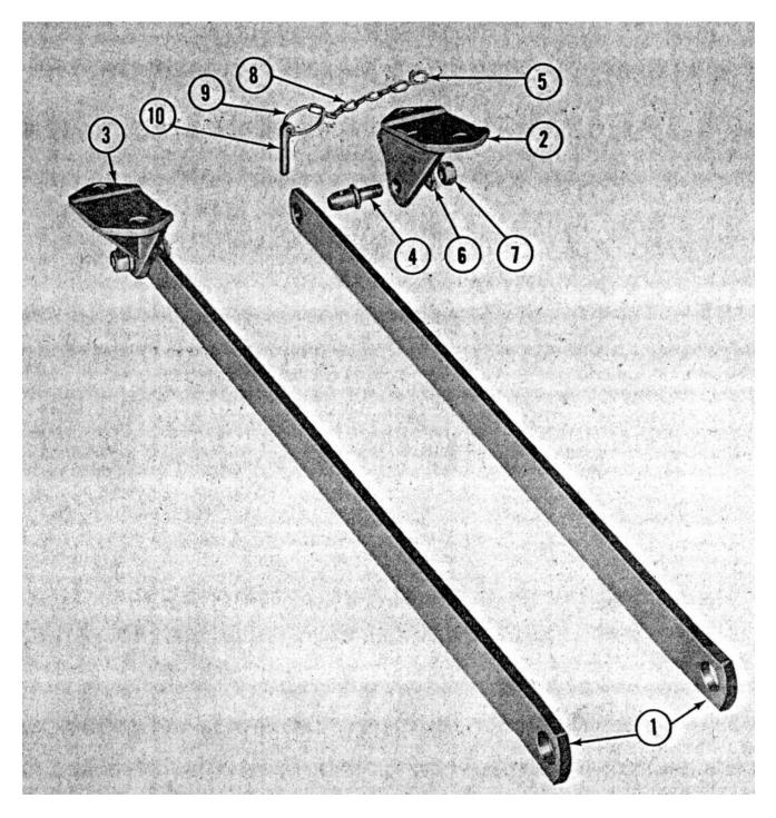
Note from the photo below that *both* stabilizer and stay bars are installed and being used with the 3-point cross-drawbar on this tractor. The stay bars will keep the drawbar from lifting, and the stabilizer bars will keep the drawbar lined up directly behind the tractor and not swing out on turns:
