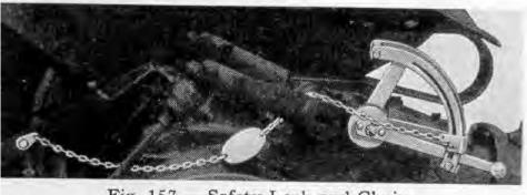
Fig. 157 - Safety Lock and Chain
