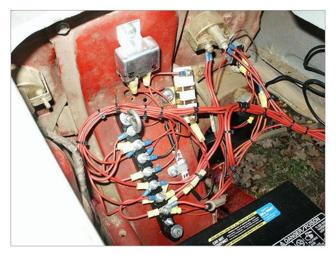
If I were doing this conversion again I would move the terminal strip to the left edge of the fire wall because there is more space between the metal and the steering gear box behind that location.
