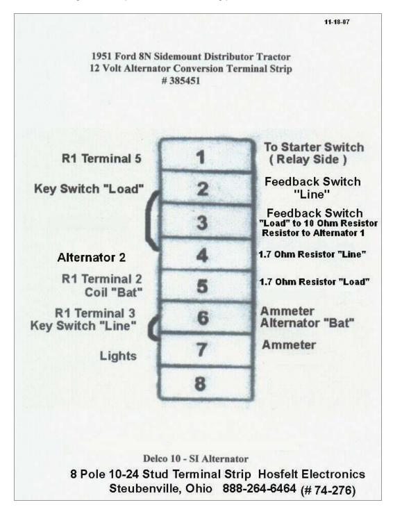
Note that terminals 6 and 7 are both connected to the un-switched positive side of the battery.
