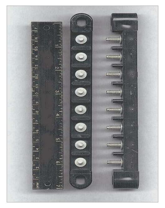
The original terminal block has been replaced with an 8 terminal phenolic stud strip that is mounted on the back side of the instrument panel. (I needed a good sharp drill for the tap holes. That is one hard piece of metal) Most of the wiring is routed through this strip. The wiring is #16 AWG and #12 AWG stranded automotive type wire. The jumpers on the strip are #12 AWG wire.
