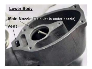
With the venturi out, remove the Main Nozzle. Use a nut driver or deep socket to get the nozzle out. Make sure that you don't cock the nut driver or socket to one side or you will bend the nozzle spout which will keep it from breathing properly when reassembled.
