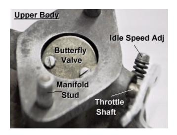
After the upper body is thoroughly clean and dry, it is time to replace the throttle shaft. 99% of old carburetors leak air around the throttle shaft and that upsets the air-fuel mixture something terrible. The throttle shaft is made of brass and is the part that wears; the throttle body bore is usually unaffected.
