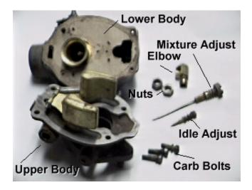
Remove the idle mixture screw/needle, spring and gasket, the power mixture screw/needle, spring and gaskets, and the fuel strainer/elbow.
