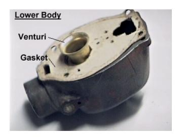
As you can see in this rebuild, the hand made cardboard gasket stayed with the lower body. For you information, this won't usually be the case. A manufactured gasket, similar to the one that comes in your rebuild kit, will be retained under the float in the upper body because of the way it is cut.
