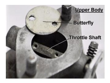
Look around the throttle shaft to see if there are any really pronounced burrs in the brass. You are about to pull the shaft out through the bore and don't need any junk scoring the bore.
