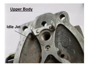
Next to the float seat is the idle jet seat. This is the jet into which the idle screw/needle fits when the carburetor is running on your tractor. Removing this tiny jet is also tricky since its bearing surface is even smaller than the float seat. Use the widest straight slot screwdriver that will fit the casting hole and fit into the idle jet slot. Same as before, keep the screwdriver from slipping and the jet will come out.
