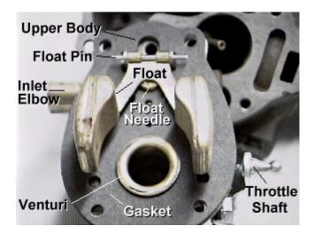
Reinstall the float seat with its round gasket and float needle in the upper body. Install the new body gasket and seat the venturi (note the dot you placed on the venturi to face the LOWER body). Reinstall the fuel inlet elbow/strainer with a new gasket and filter. Place the float over the float needle and insert the steel float pin through the ears in the casting to retain the float.
