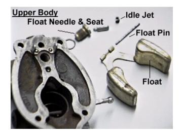
Assuming that your rebuild kit has the replacements, discard the old float needle, seat and gasket, and the old steel float retaining pin. Retain the idle jet (seat) and the float, and, of course, the upper carburetor body.
