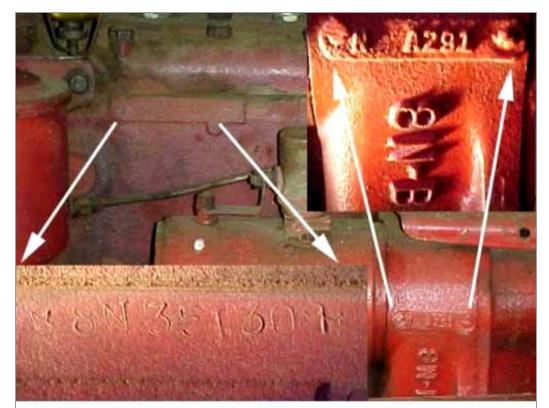
Serial number \*8N351309\* Engine casting date A291 where A= January; 29 is the day - 29th; and 1 is for 1951 Note: the serial number and engine block casting date are on the SAME casting so they can not be separated like other castings can from the original tractor.
