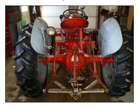
Since I mow frequently with an 8N I decided to make this seat fit an 8N. The first step was to set it on the 8n and see if it was even possible. The rear shock mount was not, due to the differences in the rear center housing the existing bracket could not be used. The coil spring mount on top of the hydraulic cover interfered with the position control lever.
