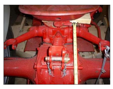
A location was determined that allowed the seat to fully compress just as it bottomed out and worked for the fully extended position. The upper mount was cut off and relocated to its new location. I had to move it from the top of its mount to the underside to clear the seat. I also moved it to the left to allow for the shock to center in the space available on the lower mount.
