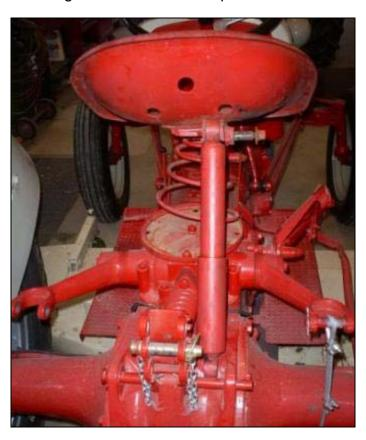
In order to use this mount on the rear end, the upper mount location had to change on the seat. I began checking new potential locations for the mount while considering the shocks extended and compressed positions. The shock measures about 18" center to center extended and about 11.5" compressed.
