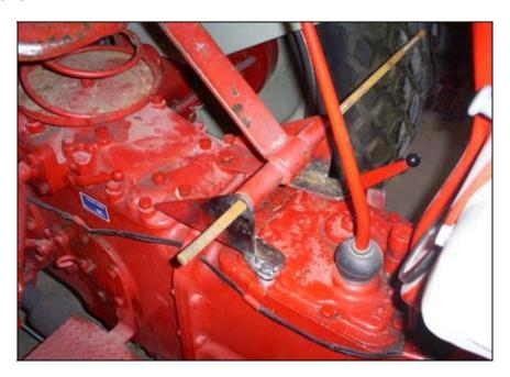
The only available location on the rear casting for the shock mount is the long pin on the pivot for the 3pt spring. I tested this as a location and it appeared ok but upon measuring the stroke of the shock the seat sat too high and would not compress down to level.
