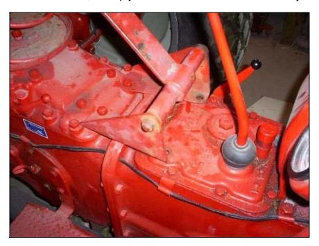
After studying the seat assembly for several evenings I figured it was a go. The hydraulic cover is roughly the same between the 2 tractors so this mounting point would stay, the seat would be built around that point.
