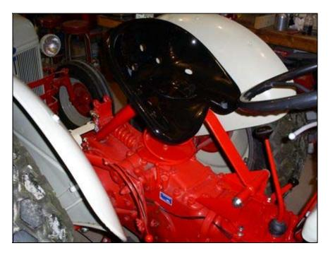
In this view you can see the notch I made in the spring mounting plate to allow for shock compression. I also removed the position control lever which is bent from the factory and straitened it. This eliminated the interference with the spring mounting plate.
