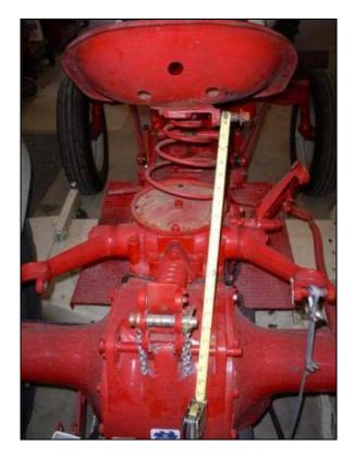
The seat was check extended and compressed looking for the right place to relocate the upper mount.
