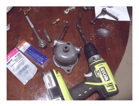
Tap the freshly drilled hole with a 1/4" x 18 NPT tap. Extreme care must be taken here to keep the tap straight and aligned with the hole, as well as keeping downward pressure. Use cutting oil. (Pot metal will shear much quicker than steel.) Tap cost \$5.29
