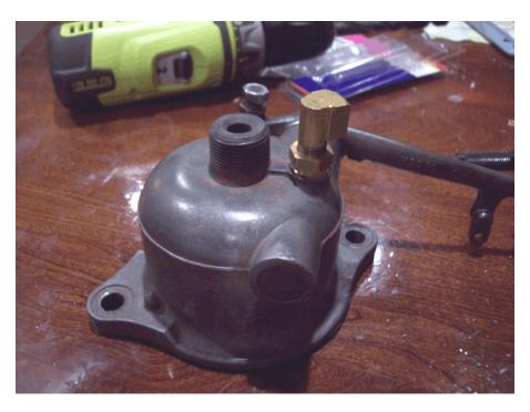
While I had the arms off my governor, it was a good time to repair the wobble that is so common with these governors. I cut a strip from an aluminum soda can, greased it and wrapped it inside the lever (9N18190 (9N, 2N) or 8N18190 (8N)) as a shim and re-assembled the governor.
