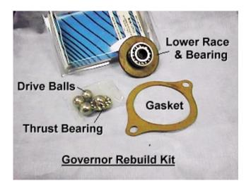
The overhaul kit consists of new steel balls, new lower race and bearing. New thrust ball bearings and gasket. The Governor fails by developing flat spots on the steel balls and corresponding wear marks on the lower race. These flat spots cause the balls to 'stick' in one position at the wear spots on the lower race rendering the Governor unresponsive to engine speed changes.
