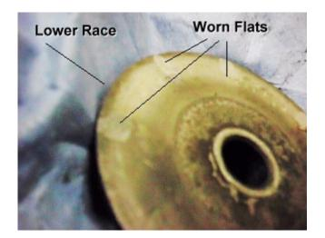
Once the lower race is off of the shaft, the wear marks become evident.
