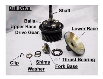
Remove the steel balls. They just fall out - nothing is holding them in at this point. Discard the thrust ball bearings. Clean the lower race of any varnish buildup.
