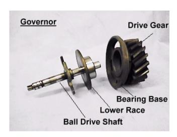
Reassembly is pretty much the reverse. Slide the new lower race and bearing from the rebuilt kit onto the ball drive shaft. Note the orientation of the lower race to the bearing. Fit the bearing base on the shaft up next to the lower race engaging the lower race bearing. Slip on the fiber spacer.
