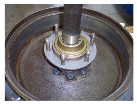
Wipe off the excess grease and put a gasket on the flange to seal the backing plate from the inside.
