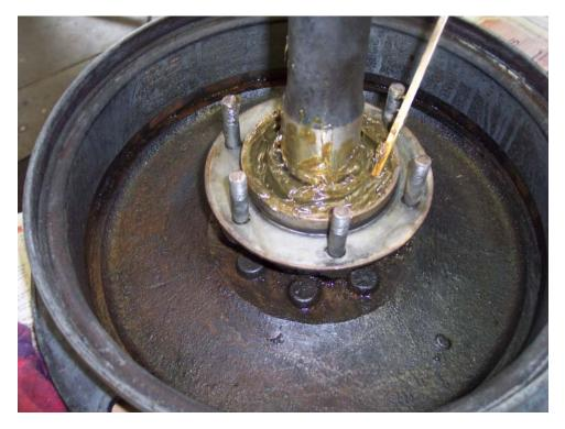
The sure seals are pretty straightforward; you first need to pack grease into the bearing assembly. I used a wood mixing stick to push grease down into the bearing. I would occasionally lift the bearing carrier and turn it several times to distribute the grease. It takes a while to complete this process but it is very important.
