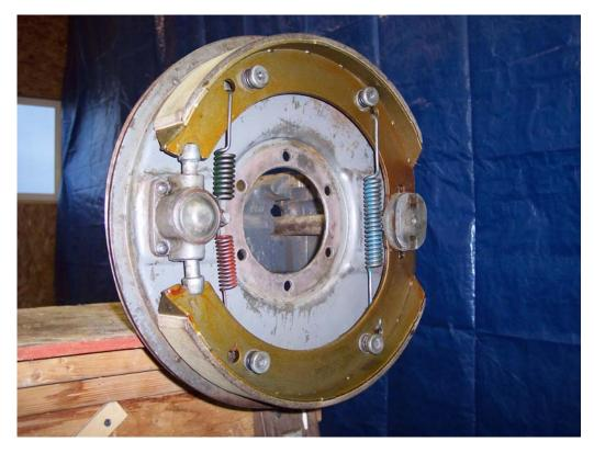
One side completed, and ready to install into the brake drum.
