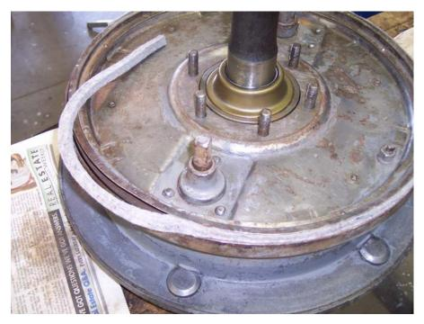
I installed new felt dust seals around the perimeter of the backing plate prior to dropping it into the drum. It is now ready to install into the trumpet.
