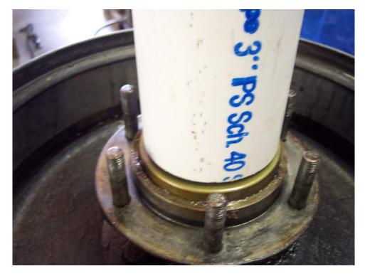
It is a little tricky doing the seal install this way because the seal wants to rock around. I stood above it and held a 2"X 4" on the top of the PVC and struck it with a hammer. I would stop and take a look as I was doing it because I didn't want the seal to go in at an angle. Once I had it started I removed the PVC and used a piece of 1' X 2" to tap the seal in evenly.
