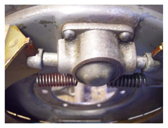
It is important the brake shoes seat into the brake shoe links. Make sure the brake adjuster is turned all the way in before putting the assembly inside of the brake drum. This is done from the other side of the backing plate.
