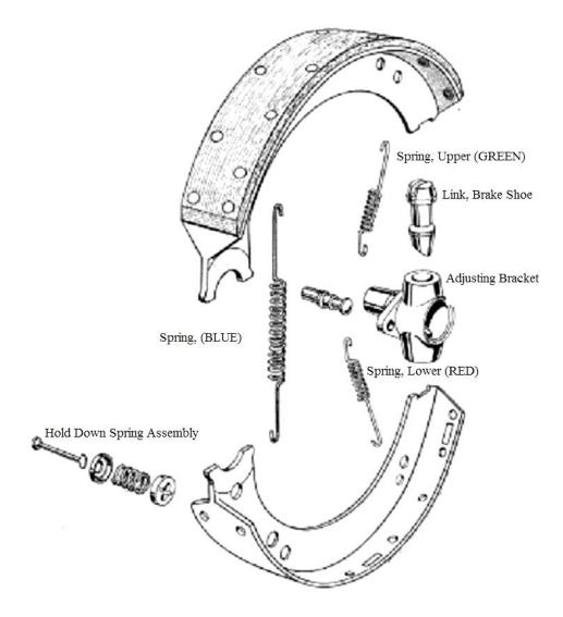
These are the parts I will be referring to. The placement of the springs is important. Since there are a right, and left brake assembly pay particular attention that the "GREEN" spring is on top when assembled.
