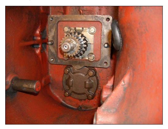
Put sealer on the rear main housing gasket and install the main housing. Make sure the selector gear is pointed the right way and is seated in the shifter fork.
