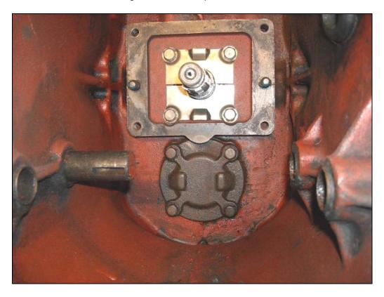
Don't forget the wires to lock the mounting bolts and install the gears and snap ring on the shaft. Use assembly lube on the gears:
