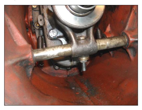
Install the springs to the throw-out bearing carrier and make sure that the clutch shaft and the carrier mates between the forks and operates properly. I always replace the throw out bearing while the tractor is split.
