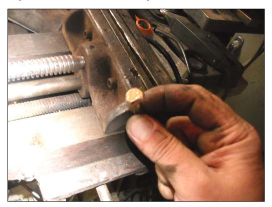
Put the throw-out bearing springs on the OD housing while you still have lots of room. With the bolt head ground, the bolt seats against the clutch fork.
