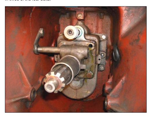
Add the 1 pint of lube (the same lube that you are using in the tractor transmission) to the Sherman OD by putting it in through the open bolt hole at the top right. Install the bolt and do the final torque of all the bolts.
