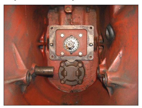
Final install of rear housing with the baffle plates:
