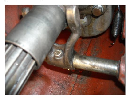
Install the washers and the lock nut. I use a long bolt with washers to keep the full diameter of the bolt in the full depth of the connection between the fork and the shaft.
