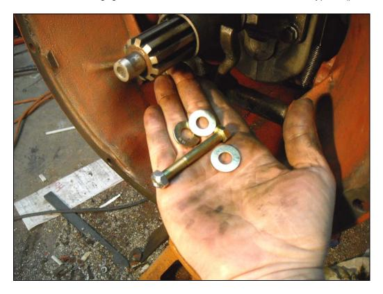
To get the head of the bolt to seat I had to grind the head on one side flush with the shank.
