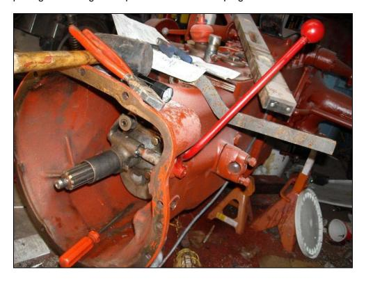
Locate the shifter arm between the two disks on the shifter rail. Then install the cotter pin on the shaft and the cross pin and cotter through the shift lever and check for smooth operation. It's a great feeling to shift the Sherman and watch the rear hubs turn in both high and normal range.
