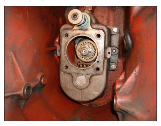
Install the shifter lever in the front housing and install the front housing on the main housing with sealer and put in three of the four bolts:
