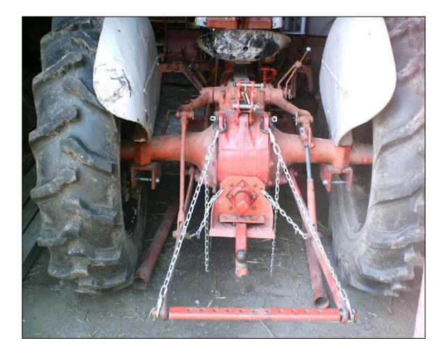
Note: Be sure to secure the excess length of chain. Do not let it hang down like pictured when you are using the tractor!
