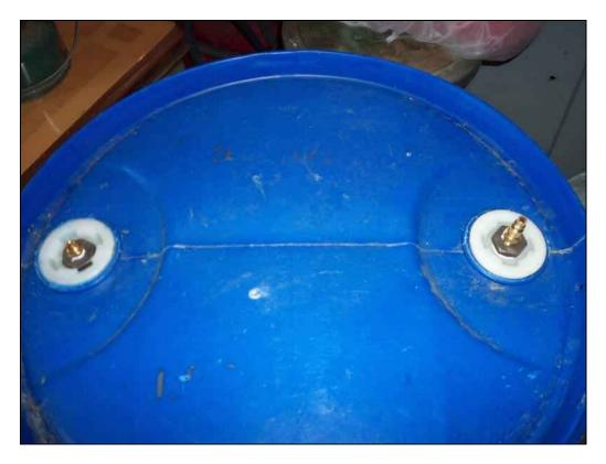
The bungs have a smaller outlet in them that is 3/4 inch pipe thread. Just cut out the inside plug. I used 3/4 to 1/2 reducing bushings and installed the copper tubing fitting into the bottom bung and about 6 foot of 1/4 inch outside diameter copper tubing. The top bung I installed a air quick disconnect fitting. If you had a place that you could put the barrel higher than the tractor, you could let gravity do its job and not bother with an air compressor.
