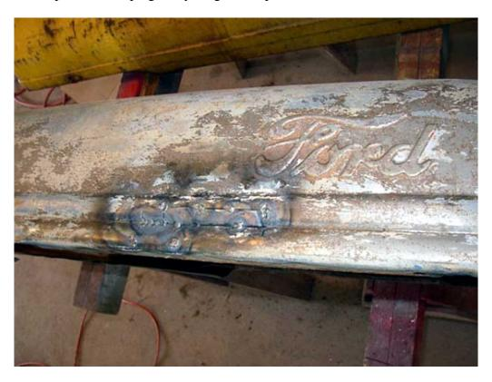
Once everything is in place and lined up, weld it in. I work in small areas and alternate allowing the metal to cool to minimize distortion. I use an acetylene torch but a mig welder would be easier to use.
