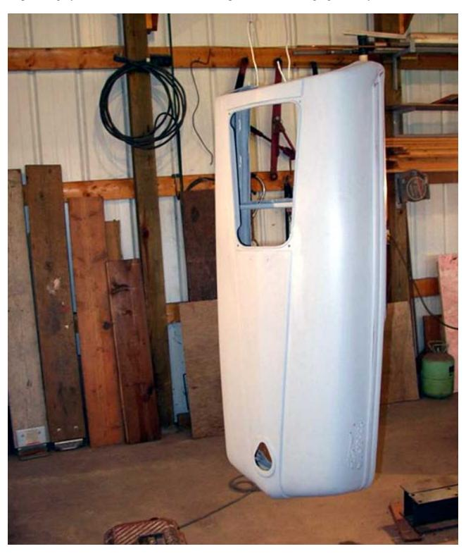
Now paint with your coating of choice following the mfg's directions. Be sure to paint inside the hood around the cross braces and along the horizontal rib.
