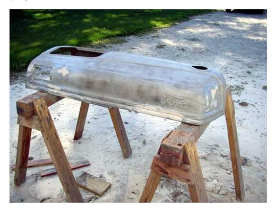
I am using automotive type primer with high solids for surface building. It has very quick dry time which allows you to sand and prime, sand and prime, sand and prime.
