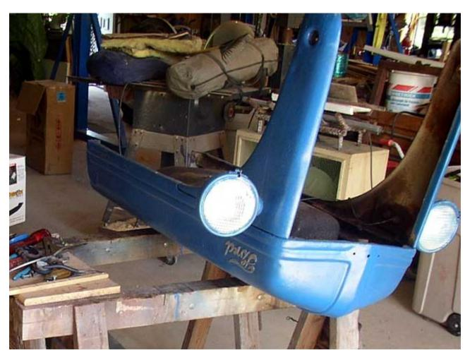
Disassemble the hood. I use paint stripper and strip the hood. Perform a close inspection and look for rust in the lower rib running along the length of the hood. They usually rust near the front and along the side near the rear cross support.
