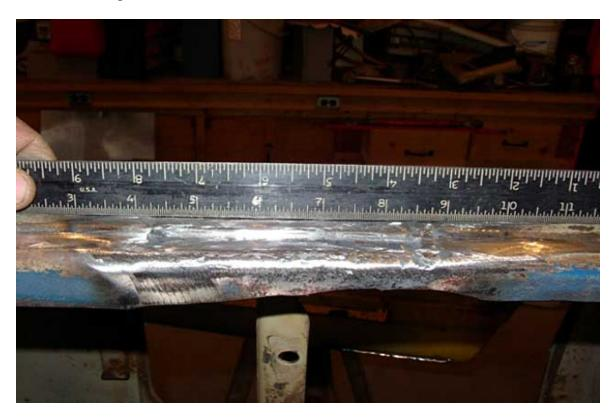
Once the repair is in, sand blast the exterior of the hood and inspect for more damage. Sandblasting has a way of locating holes in the hood. I also mark dents on the inside before blasting as they can be hard to locate after the hood is blasted.
