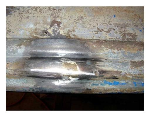
Once sandblasted you can use the filler of your choice and fill it in. Be careful to restore original lines etc. You can also work on hammering out those dents and using Bondo to you liking. Once I have my repairs filled to my liking, I prime the outside of the hood with red primer. With Bondo I use 80 grit sandpaper, followed by 150 grit, followed by 220 grit and then primer.
