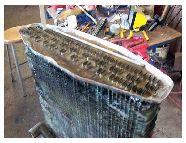
There are exactly 100 tubes in this radiator. Also notice that there are more tubes in the front of the radiator than in the center or rear. Also the rear has more tubes on the right than on the left.
