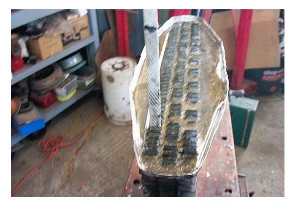
Then I took the radiator to the laundry tub and scrubbed it and ran hot water with detergent (Purple Power) through the tubes. After a good cleaning, I soldered the top tank back on and soldered on a filler neck.
