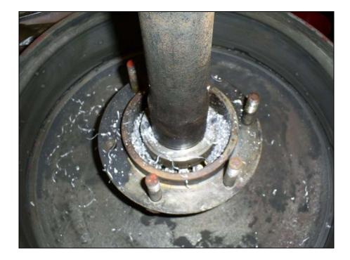
Cut the collar with a chisel where you drilled. The collar is soft and easy to break at this point. Once broke its easily removed.
