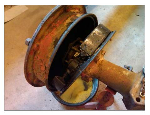
With the drum removed, make note as to the color of the springs and their locations. The proper location is green on top, red on bottom. The large spring is blue. I prefer to clean the assembly before disassembly. Once clean, remove all the parts and set aside.
