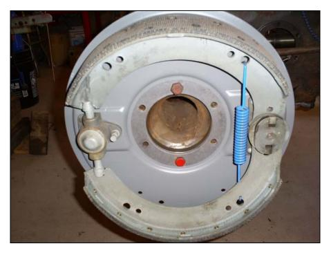
Add the remaining springs, Green on top, red on the bottom. Check to see that the brake pedal and adjuster expand the brakes. Make sure both are retracted. Once complete remove the assembly and set aside.
