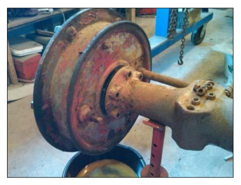
The brake backer plate may come out with or without the brake drum and it doesn't matter. I chose to separate the backer plate from the drum as it comes off the tractor as It's a little lighter that way. Have a long bolt or something handy to shove through the axle and backer plate if you wish to leave it on the tractor.
