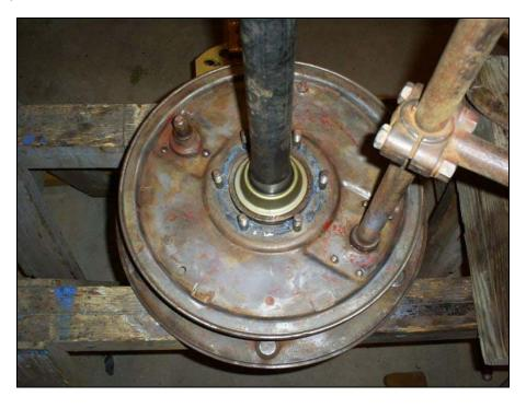
Slide the axle and brake backer plate into position on the tractor, make sure the brake cross shaft is seated in trumpet casting and tighten the 6 nuts. You may have to rotate the hob to get the axle to slide into the differential. You can see the silicone oozing out, this should be a very good seal. Test to see that the hub still rotates and that the brake works. You will adjust the brakes later.
