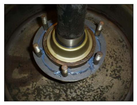
Slip the brake backer plate with the brakes installed into the brake hub.
