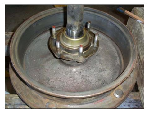
Using the proper number of shims (gaskets) determined from setting the axle end play, add them to the sealing areas. I used a small bead of silicone sealer on both sides of each gasket as unfortunately I expect to back in here again someday.
