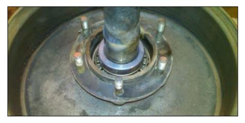
Before the seals are installed on the axles, or the brakes on the backer plates, it's time to set the axle end play clearance.
