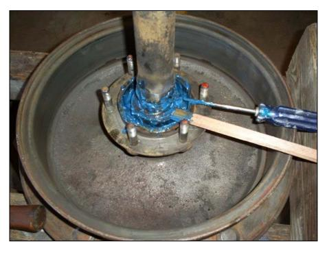
Even if you installed the original axle seals install a set of Sure Seals. They can be tricky to get started. I've found that using an old axle bearing cup is just right to place on the seal and carefully tap with a hammer to get the seal started strait. An alternative method is a 30" long piece of 3" PVC pipe slipped over the axle and driven with a block of wood. Avoid beating on the seal directly with a hammer.
