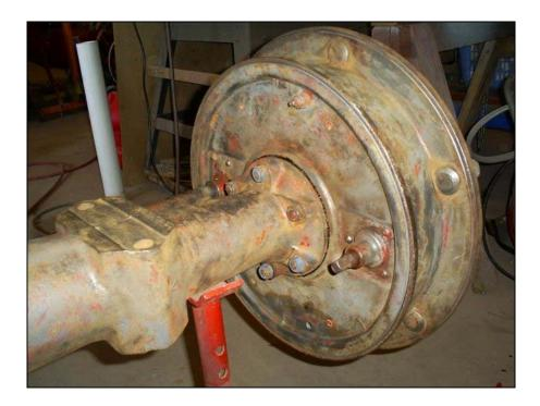
Stand back and admire your work. The hub is complete. You will need to run the tractor and adjust the brakes several times as the pads seat in and the high spots wear off. Remember to fill the hydraulic/transmission cavity with the correct oil and don't overfill. The capacity of oil far exceeds what is needed to operate the hydraulics so running the level high just adds to the oil present at the axle seal. Running the oil a bit low is far better than a bit high.
