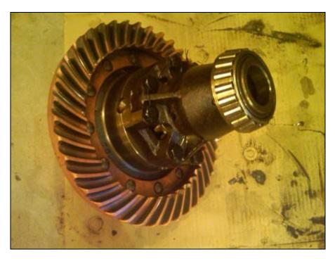
Replace the actuator shaft bushings. They are inexpensive and likely worn out. It's best to do these off the tractor as its possible to drive the plug in the hole out which leaves it under the differential. In manufacturing the hole was bored then a steel plug was inserted from the back. Guess how I learned this?
