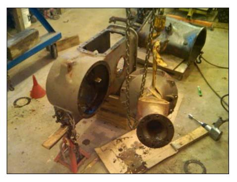
With the left trumpet off, reach in and remove the differential. This is another very heavy part. Take care not to drop it. Place several layers of heavy cardboard on the floor in case you do. Once out inspect the ring gear, bearings, the bolts, and the rivets that fasten the ring gear to the carrier. Broken rivets are not uncommon and there are bolt kits available to replace them.
