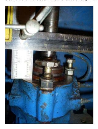
From here I lightly lubricated the new seal and reinstalled the upper casting with the new seal. It dropped onto the shaft and stopped at what I believe is the Speedi-Sleeve where it required just a little force to go on down.
