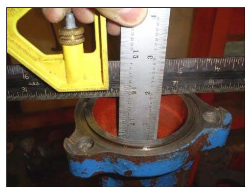
Here's a picture or the new seal. Note the bottom of the seal goes towards the lower steering assy.
