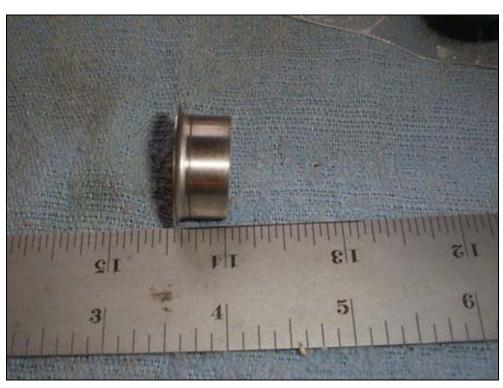
After doing some math I determine where the Speedi Sleeve needs to be installed. The photo shows the marks for the installed top of the sleeve, center of the lip seal lip, the bottom of the usable Speedi Sleeve and the bottom of the Speedi-Sleeve prior to removing the lip.
