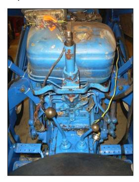
Once the upper casting is removed the lower steering assembly is visible along with the steering shaft that the seal runs against.
