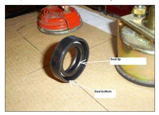
In this picture, the area where the seal mates to the shaft is indicated with a white arrow. It's easy to see the pitting and rust just above the seal area. It's important to note that the steering shaft moves up and down approx 1/8" from center during normal operation. It's likely that in this case when the shaft drops the seal lip is on the pitted area which is responsible for premature seal failure.
