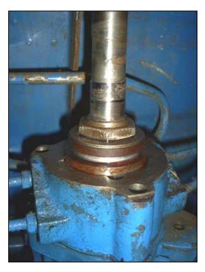
This is a picture of the Speedi Sleeve that cane with the kit. It's a very thin machined piece of Stainless steel that provides a new sealing surface without having to re-machine the shaft. It has a flared collar to aid installation that will be removed when completed. The kit comes with a bigger sleeve that fits over this one that you drive against to move the Speedi-Sleeve into position. Notice the groove on the left side near the flair; this is where the flair breaks away when installed.
