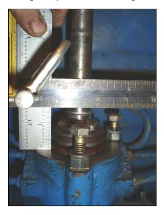
After driving the Speedi Sleeve to the proper location, I removed the flared lip and did a final check, if I've done the math right, the lip on the new seal will land exactly in the middle of the new Speedi Sleeve. Instructions for installing the Speedi-Sleeve were in the seal kit I purchased through YT.
