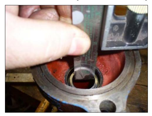
This is a measurement of the casting with the old seal removed. We need to subtract the distance from the surface of the seal to the lip.
