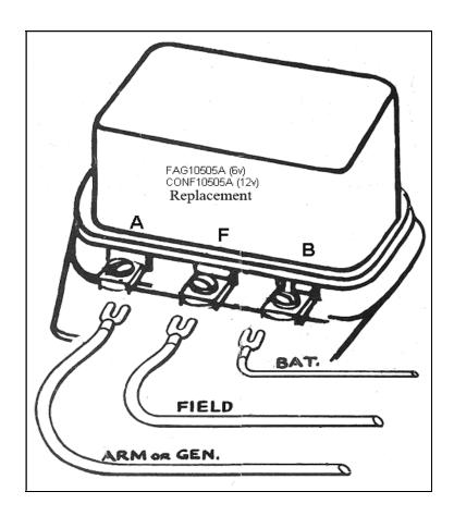
Installing a regulator is easy - but wrong installation can ruin a new regulator in a few seconds.
