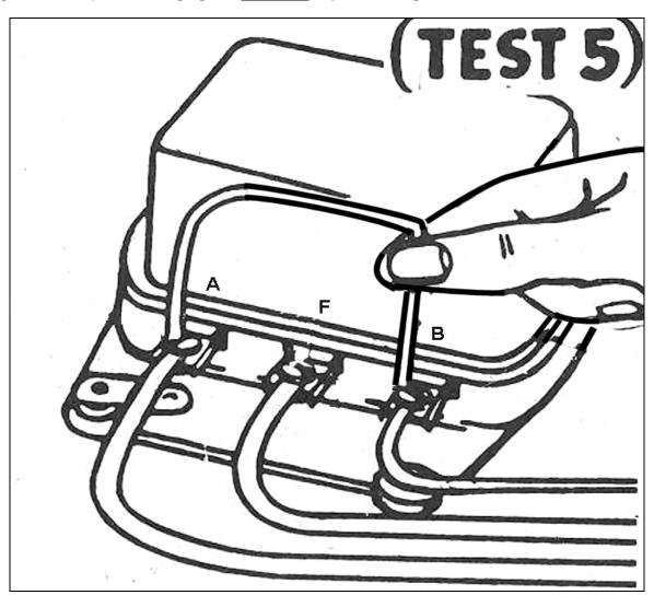
(6) If test 5 does not correct trouble, make this test.
