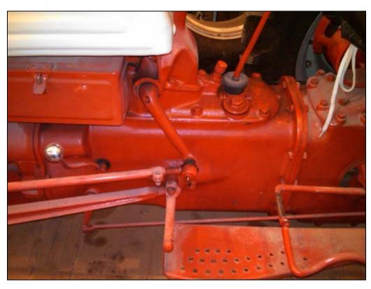
This is my 1940 Ford 9n and these steering sectors are properly timed. These arms a little ahead of the rear bolt for the radius rods. This tractor has re-production radius rods that are slightly longer than stock rods.
