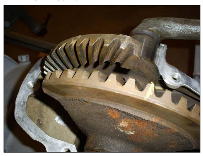
After failing the method mentioned in the book the first thought I had was to find the center of the gears, center them in the lower casting, and set the top column on. It sounds easy enough. Both gears were examined and the center of the gears for these is a tooth in the middle. The center was marked on both sectors.
