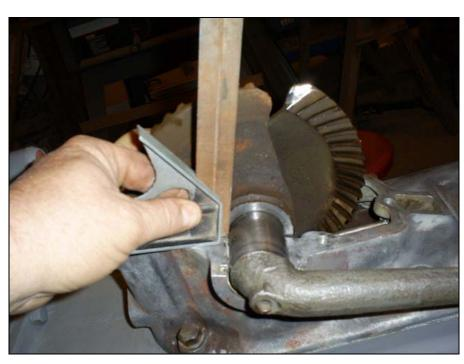
With the I&T procedure out for good it was back to landing the upper column in the correct place. Reviewing the previous failures I would need a way to hold the sectors in place as the column is lowered which allows the pinion to rotate into place. I found some wood wedges in my scrap box and tried a better way to secure the sectors. You can't provide much interference as the sectors will pop out of the lower casting.
