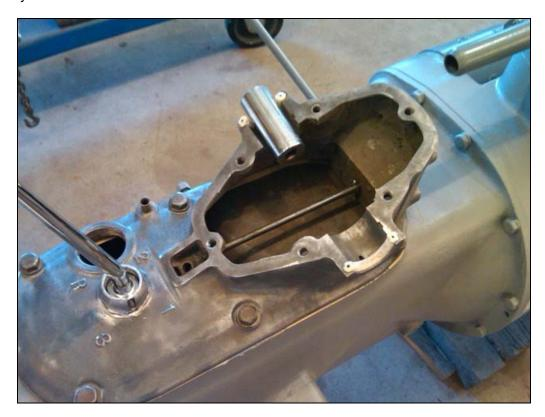
The rope ends are cut slightly higher than the mating surface using a sharp knife producing a clean cut. I cut mine slightly higher one casting and flush on the other.
