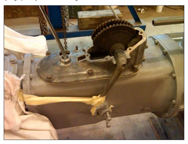
Attempt #3 was to modify the gear castings so that the I&T manual procedure could be followed. Working carefully with a grinder I added the last tooth and provided relief so that the pinion could rotate out of the sector as described in the manual. The gears are cast iron and are easily modified with a grinder. While not perfect this position is only used for timing, not steering.
