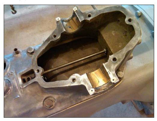
While not the best picture I used a small dab of Ultra Gray Silicon on the rope ends and a very sparing amount of Permatex #2 on the remaining surfaces, both sides of the gasket. I like to use a matchstick for applying small amounts. Not everyone will agree but I think of sealer as cheap insurance against leaks. In a perfect world the castings would be machined perfectly flat and the parts would not distort when tightened but that's not where we are with 70 year old parts.
