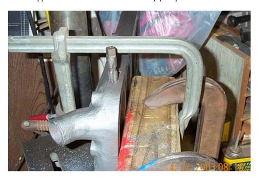
This is the end result. The sensor fits good. The head material is 3/16" to 1/4-inch thick in this spot. The head is set loose on the block. I turned the engine over and watched for any movement of the head, all is well with that, also.
