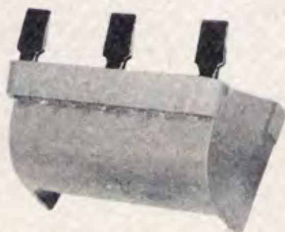
Top view of alternate bucket with teeth set for 12" cut.
