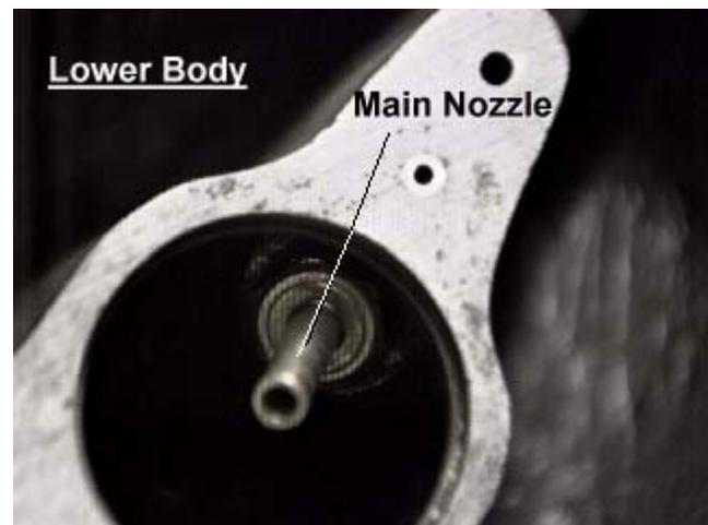
Set the discharge Main Nozzle aside. Discard the little round gasket, after checking that its replacement in the rebuild kit is the correct size.
