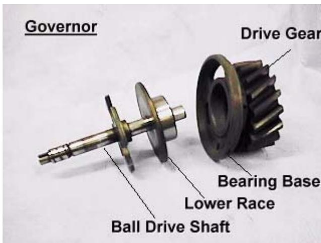
Reassembly is pretty much the reverse. Slide the new lower race and bearing from the rebuilt kit onto the ball drive shaft. Note the orientation of the lower race to the bearing. Fit the bearing base on the shaft up next to the lower race engaging the lower race bearing. Slip on the fiber spacer.
