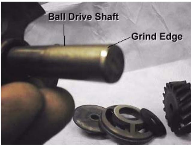
Once the lower race is off of the shaft, the wear marks become evident.
