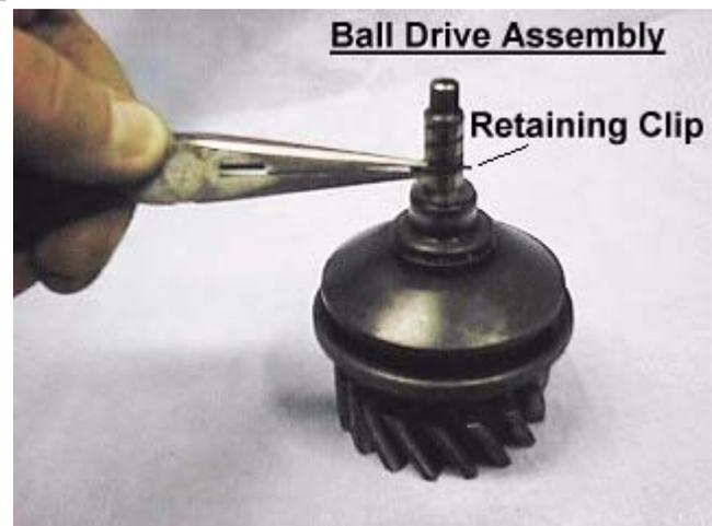
Remove the steel balls. They just fall out - nothing is holding them in at this point. Discard the thrust ballbearings. Clean the lower race of any varnish buildup.
