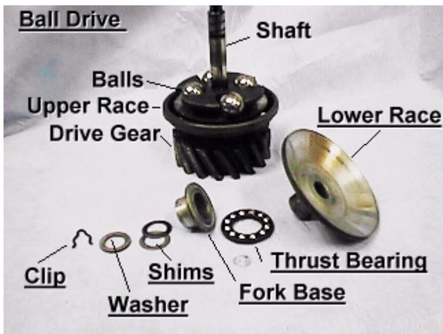
Examine the steel balls for flat spots, and the upper race for corresponding wear marks. If the steel balls are completely round and smooth and the upper race is free from any wear marks, consider other causes for the Governor not being responsive, such as binding in either of the external arms, broken or maladjusted spring, or broken drive gear. Renew as necessary. Replace the steel balls and race in any event.
