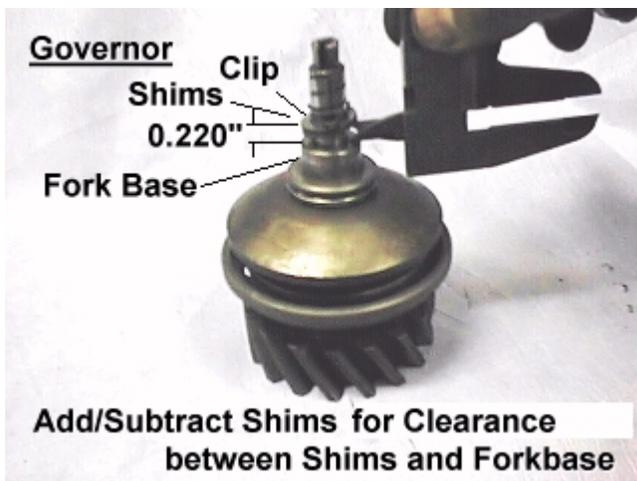
The adjustment of the thrust shims on the shaft is straight forward. With the ball drive assembly resting on the drive gear face, push down on the fork base while lifting up on the stack of shims under the washer against the clip. The distance between the top of the fork base and the bottom of the bottom shim above it should be 0.22" (less than 1/4").
