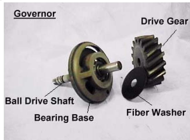
Tap the face of the drive gear with a dead blow hammer until it is seated flush with the end of the drive ball shaft. Make sure the lower race and bearing spin freely on the shaft
