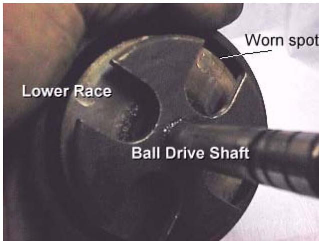
Looking down the Drive Ball Shaft towards the drive gear, with the steel balls removed, it is possible to easily identify wear marks on this lower race. It will be replaced, and is the cause of this Governor sticking.
