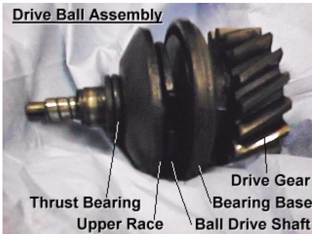
From left to right, Ball Drive Shaft Proofmeter drive end, retaining clip, washer, shims, fork base, thrust ballbearings, upper race, steel balls, ball retainer, lower race, bearing base, fiber spacer, and drive gear.
