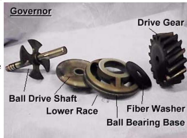
Beating on the end of the shaft with a drift will deform the shaft end somewhat. Grind a small chamfer on the end of the shaft to make reassembly easier.
