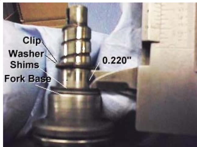
When the thrust measurement is right, reinstall the ball drive shaft into the Governor housing. Hold the bearing base against the housing and ensure that the shaft spins freely without binding or grinding noises.
