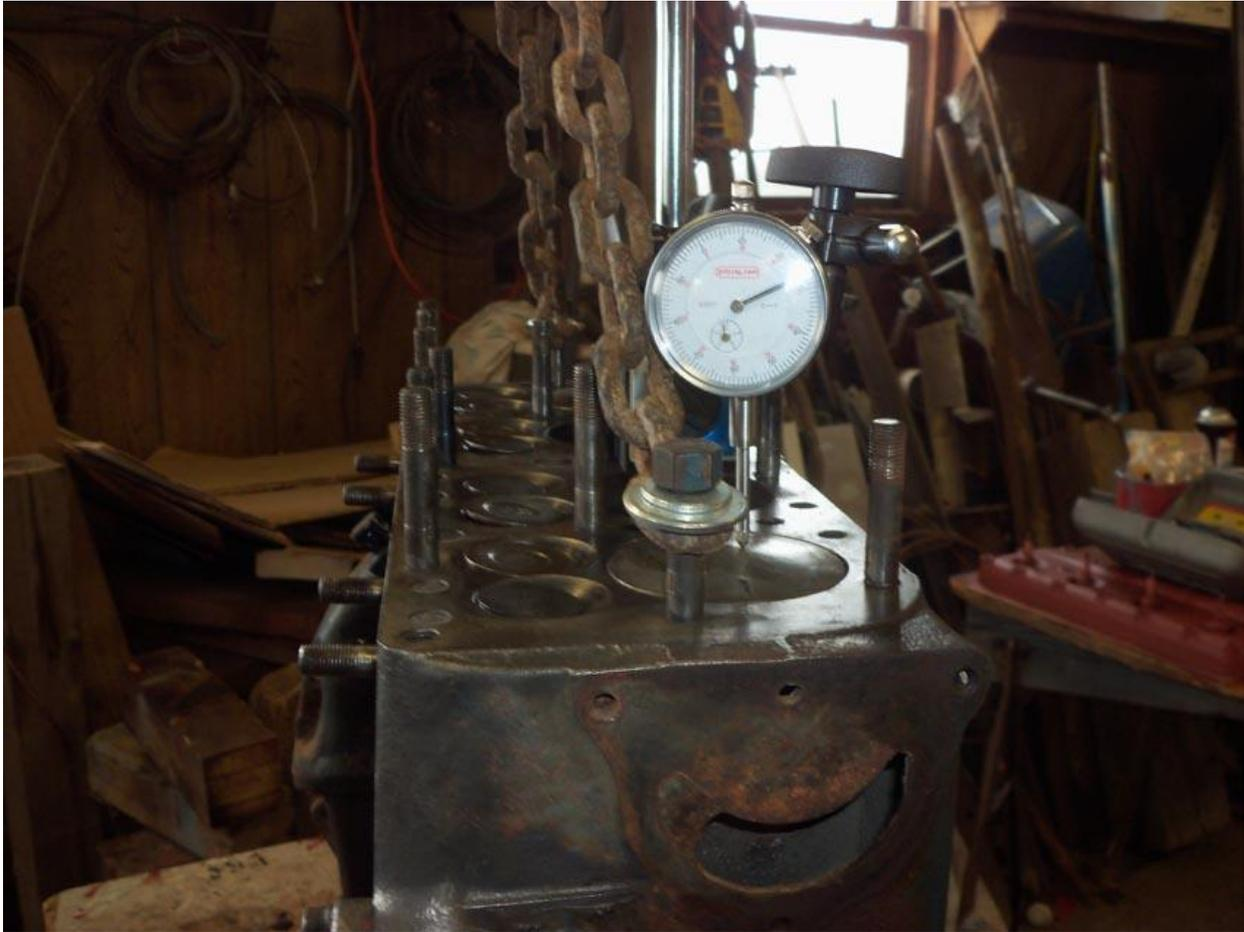
I used a Dremel tool to add marks to the front pulley and engine block. By measuring the circumference of the pulley and dividing that by 360°, I found the distance for 1° and multiplied that to get the measurements for the other marks. I used a dressmaker's cloth measuring tape to take the measurements.
