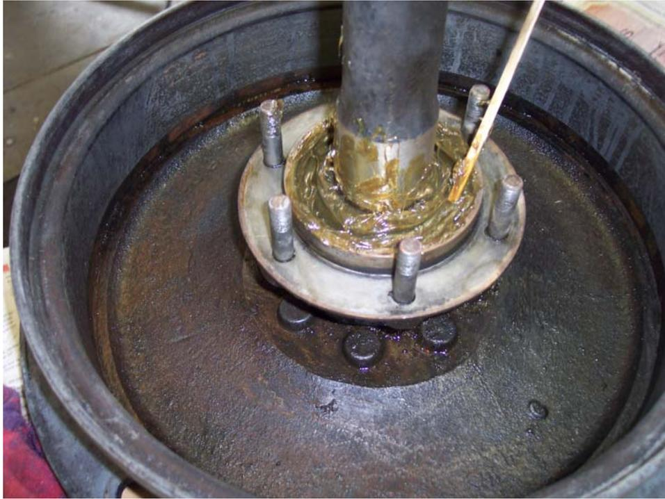
The sure seals are pretty straightforward; you first need to pack grease into the bearing assembly. I used a wood mixing stick to push grease down into the bearing. I would occasionally lift the bearing carrier and turn it several times to distribute the grease. It takes a while to complete this process but it is very important.
