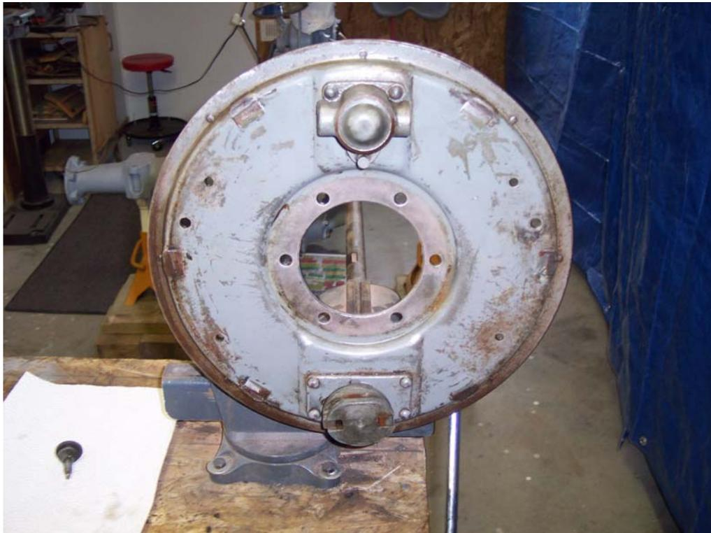
Using the brake actuator rod as a clamping surface I stripped the backing plate down as far as I could. I cleaned off the remaining crud and lubricated the adjusting bracket and made sure it would rotate. My adjustment brackets were both froze up when I disassembled the backing plate. It may not be a needed step on your assembly, just make sure not to over-do it with the oil and clean off any excess.
