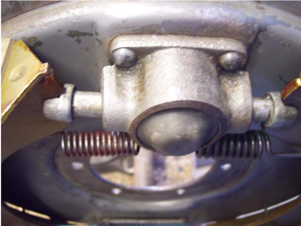
It is important the brake shoes seat into the brake shoe links. Make sure the brake adjuster is turned all the way in before putting the assembly inside of the brake drum. This is done from the other side of the backing plate.
