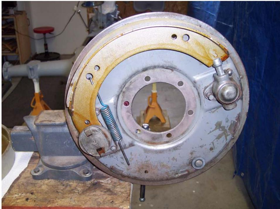
"This picture is for the purpose of showing the actuator rod pivot point, and blue spring location. The sequence picture was to blurry to show."
