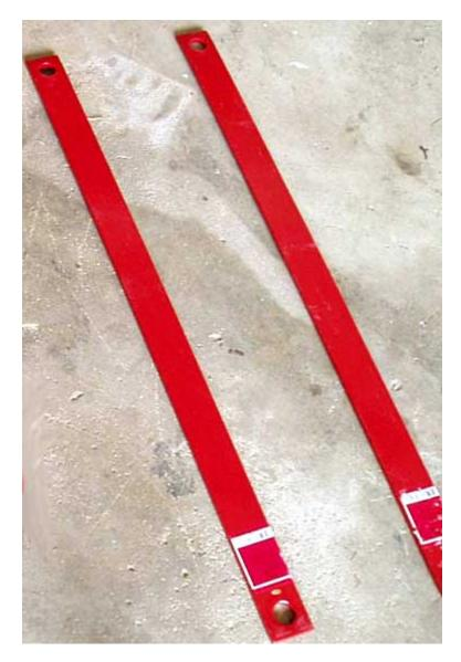
• One stabilizer bar (at a minimum), two to stabilize both lift arms. Typically, one end of the stabilizer bar is flattened; the other will have a slight curve outward. The flat end attaches to the short, Category-1 pin attached to an L-bracket. The curved end attaches to the lift arm pin, with the curve facing outward, away from the tractor.
