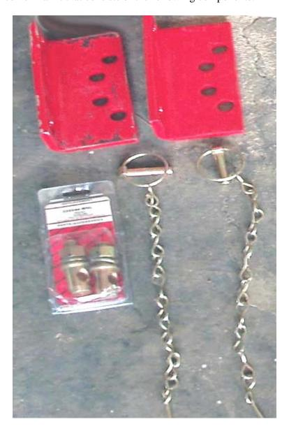
• One L-bracket per stabilizer bar to be installed. It is installed under a rear axle, using the same bolts that attach the fender to that axle. Note: the existing bolts that attach your fender will most likely be too short
