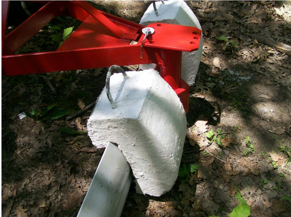
bent reinforcement rods for handles and to reinforce the “hooks” that fit over the top edge of the blade and the tough part of the job is done.
