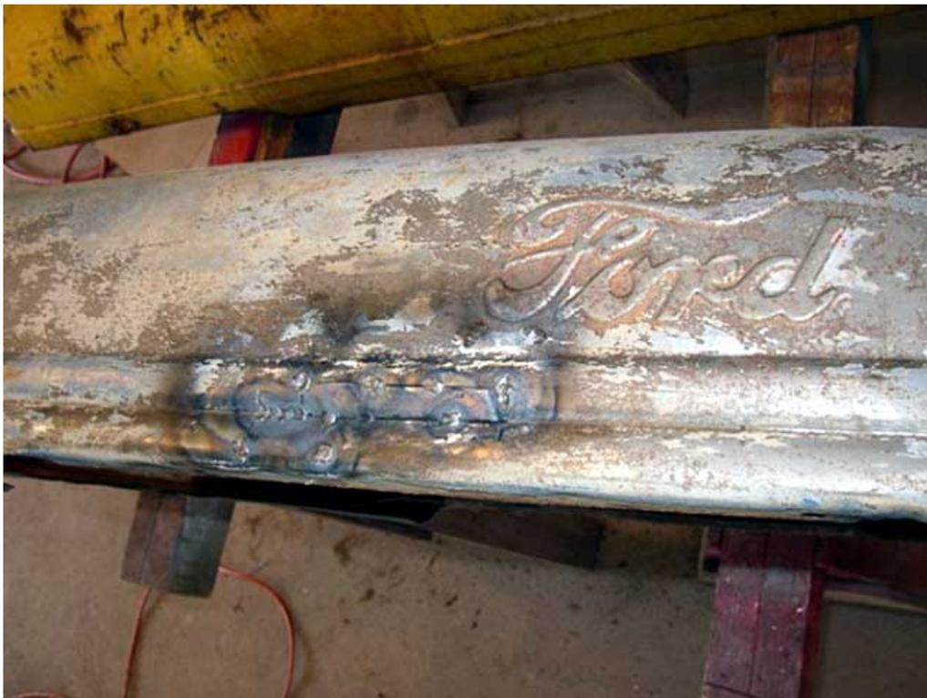
Once everything is in place and lined up, weld it in. I work in small areas and alternate allowing the metal to cool to minimize distortion. I use an acetylene torch but a mig welder would be easier to use.
