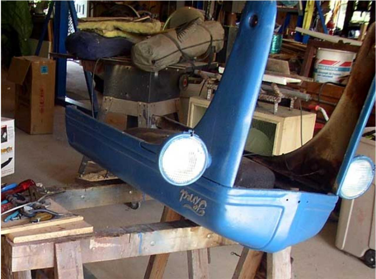
Disassemble the hood. I use paint stripper and strip the hood. Perform a close inspection and look for rust in the lower rib running along the length of the hood. They usually rust near the front and along the side near the rear cross support.
