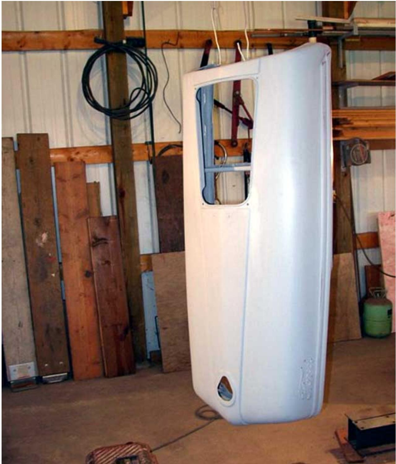
Now paint with your coating of choice following the mfg's directions. Be sure to paint inside the hood around the cross braces and along the horizontal rib.
