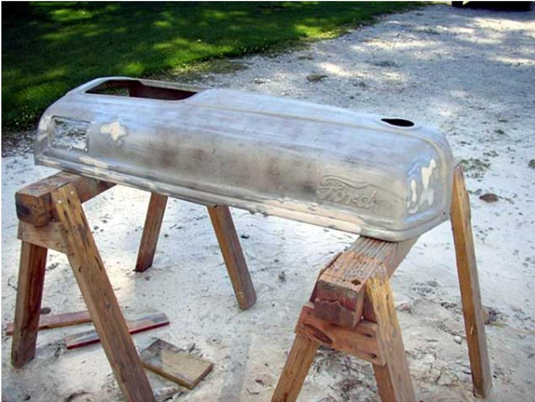
I am using automotive type primer with high solids for surface building. It has very quick dry time which allows you to sand and prime, sand and prime, sand and prime.
