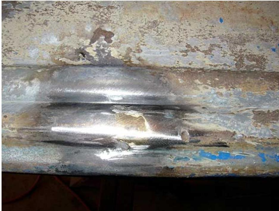
Once sandblasted you can use the filler of your choice and fill it in. Be careful to restore original lines etc. You can also work on hammering out those dents and using Bondo to you liking. Once I have my repairs filled to my liking, I prime the outside of the hood with red primer. With Bondo I use 80 grit sandpaper, followed by 150 grit, followed by 220 grit and then primer.
