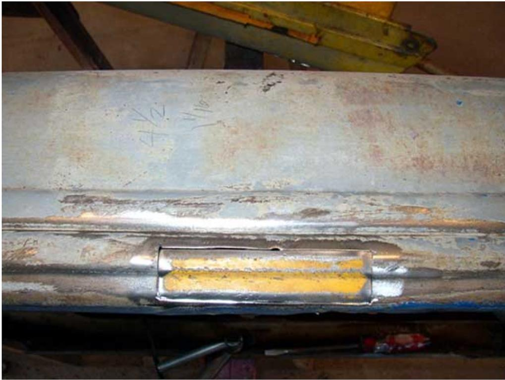
Here is another repair to the other side. Cut out the old damage first and make pieces to weld back in:
