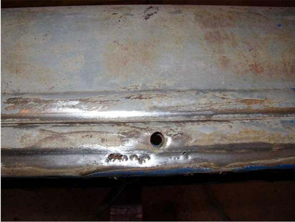
Cut out the damaged area using a cutoff tool:
