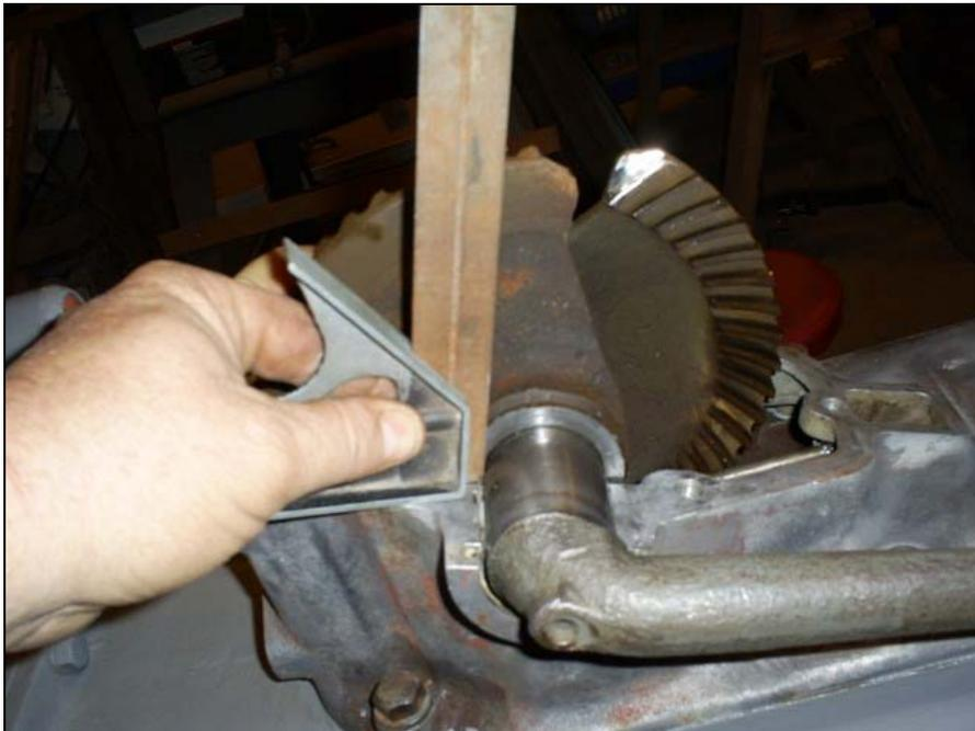
With the I&T procedure out for good it was back to landing the upper column in the correct place. Reviewing the previous failures I would need a way to hold the sectors in place as the column is lowered which allows the pinion to rotate into place. I found some wood wedges in my scrap box and tried a better way to secure the sectors. You can't provide much interference as the sectors will pop out of the lower casting.
