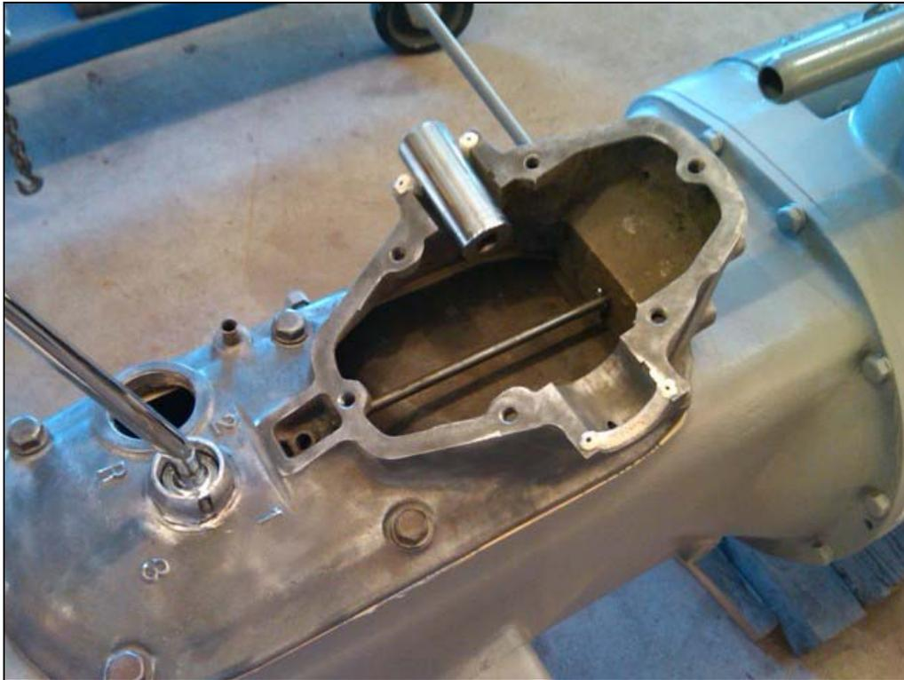
The rope ends are cut slightly higher than the mating surface using a sharp knife producing a clean cut. I cut mine slightly higher one casting and flush on the other.
