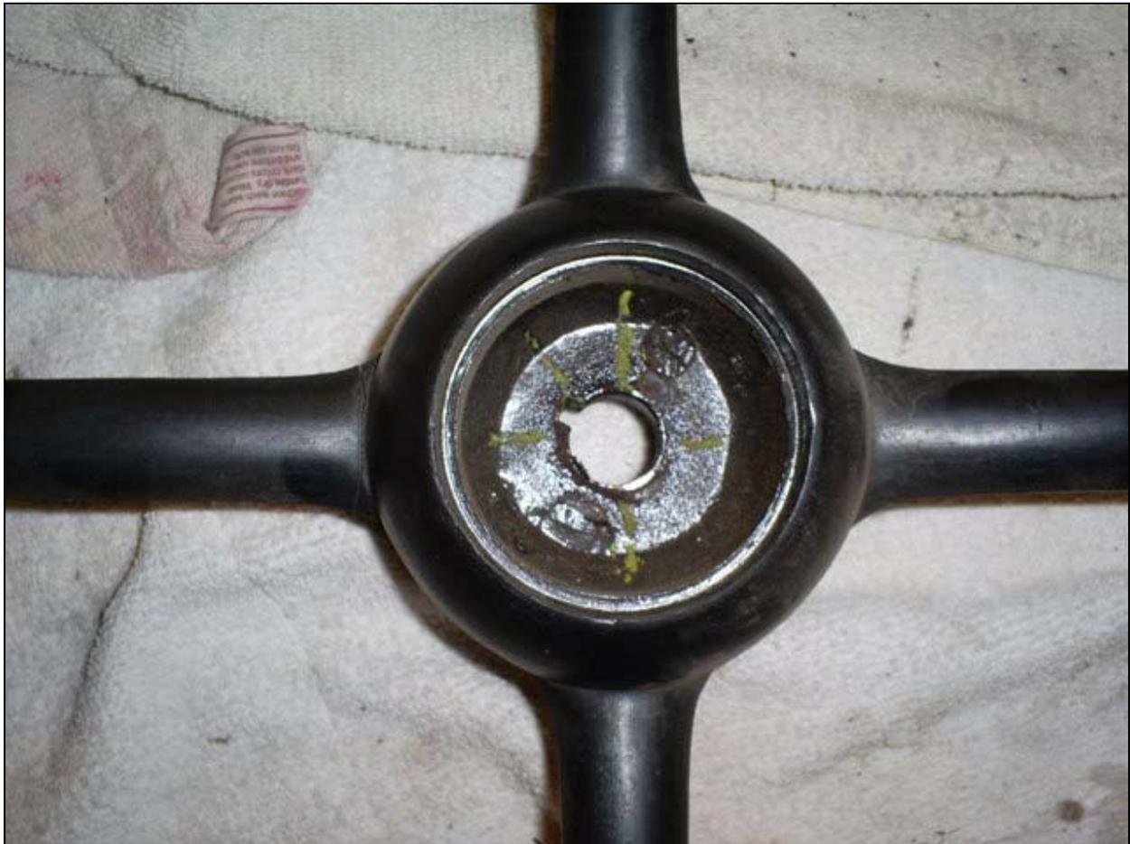
I made multiple attempts to "land" the upper steering column in the center of the gears while holding the sectors still, while allowing the steering shaft to rotate upon engagement, and having the key end up in the proper location. While it should work this procedure did not produce a repeatable outcome and cost me a set of gaskets and seals from the repeated attempts to get it right.
