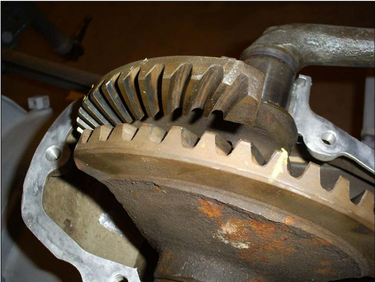
After failing the method mentioned in the book the first thought I had was to find the center of the gears, center them in the lower casting, and set the top column on. It sounds easy enough. Both gears were examined and the center of the gears for these is a tooth in the middle. The center was marked on both sectors.
