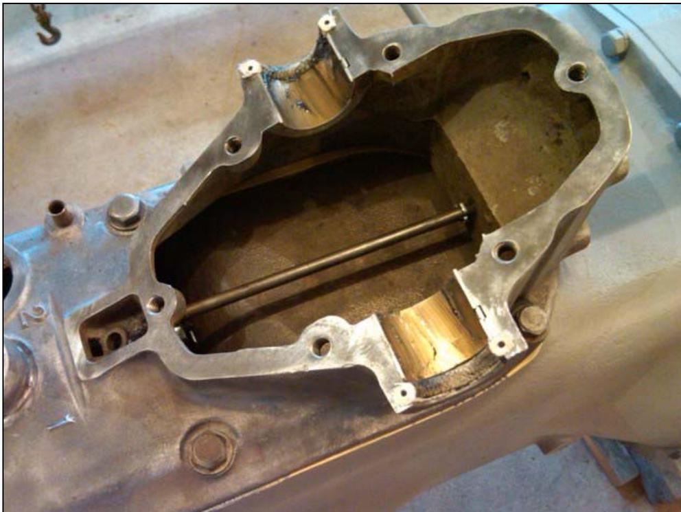
While not the best picture I used a small dab of Ultra Gray Silicon on the rope ends and a very sparing amount of Permatex #2 on the remaining surfaces, both sides of the gasket. I like to use a matchstick for applying small amounts. Not everyone will agree but I think of sealer as cheap insurance against leaks. In a perfect world the castings would be machined perfectly flat and the parts would not distort when tightened but that's not where we are with 70 year old parts.
