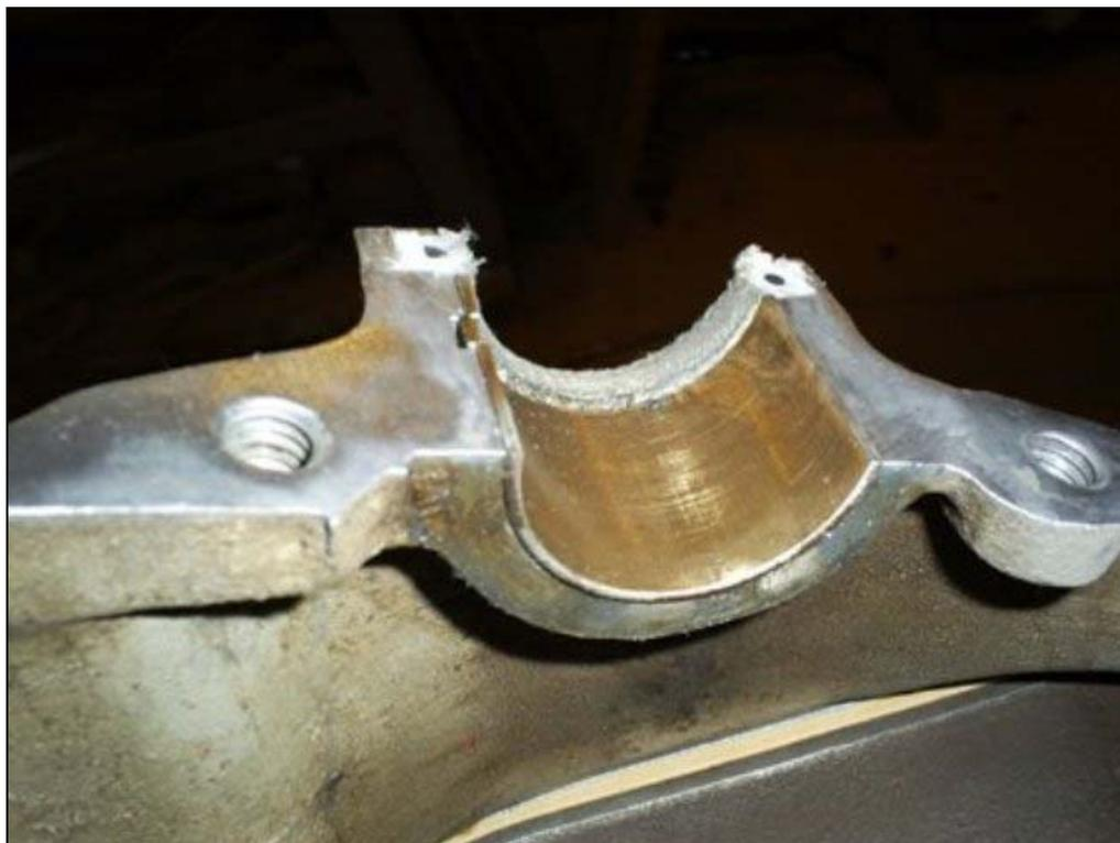
New gaskets can be made. I ruined my first new set and made another out of a similar thin slick paper like the originals. The paper in the I&T manual is very similar to the new gaskets. Hold the paper against the surface while going around the casting with a ball peen hammer carefully striking the edges of the casting creating lines and holes.
