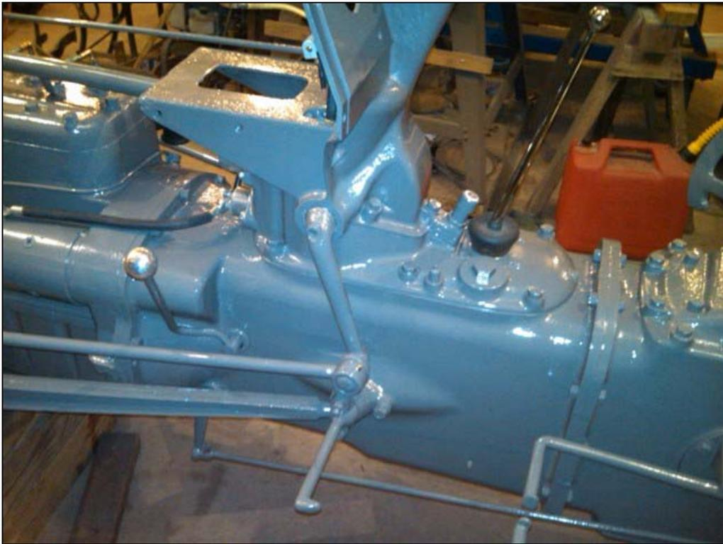
Here the tie rod ends are seen adjusted in the middle of their adjustment. While the amount of adjustment needed may vary by gear/rod set this would be an acceptable amount of adjustment.
