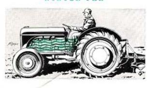
78-8600 • Pull-type fan sends warm air back toward operator for more comfort in cold weather operation. Fan is 4-blade type, easy to install.
