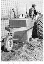
Easy to dump—A pull on the handle trips the toggle linkage and the scoop automatically dumps to vertical, then returns to operating position. The pivoting mast on the fully mounted model lets bucket rotate 32 degrees beyond normal vertical dump, a handy feature for levelling dumped loads.
