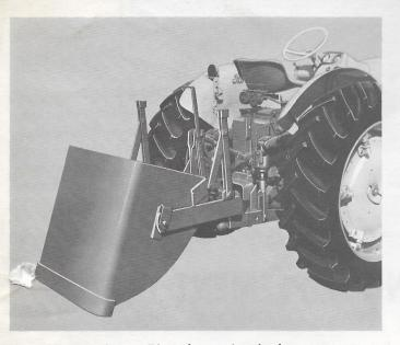
**Easy to dump**—Pivoted mast lets bucket rotate 30 degrees beyond normal vertical dump. This permits convenient levelling of dumped loads and easy dumping of difficult materials. In full raise position, it provides a high 31-inch clearance.
