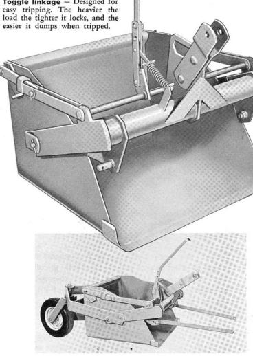
Angled cutting edge — Five degree angle provides suction similar to plow share. Makes digging easier. Full 37½-inch cutting edge of long wearing high carbon steel has continuous weld across width of scoop.
