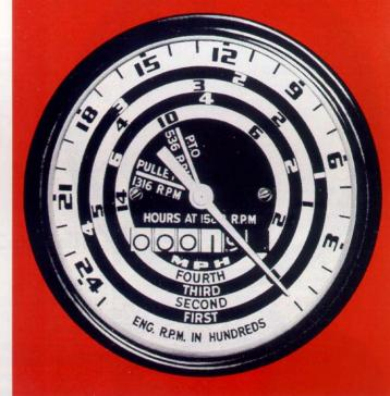
\*8N Ford Tractors with serial numbers beginning at 8N-273178 can be equipped with the Proof-Meter by installing a conversion kit consisting of a Proof-Meter, and new instrument panel. Other 8N Tractors require the above plus a new governor (part number 8N-18204-B).
