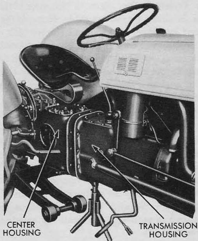
Fig. 59—Aligning Transmission Housing and Center Housing
