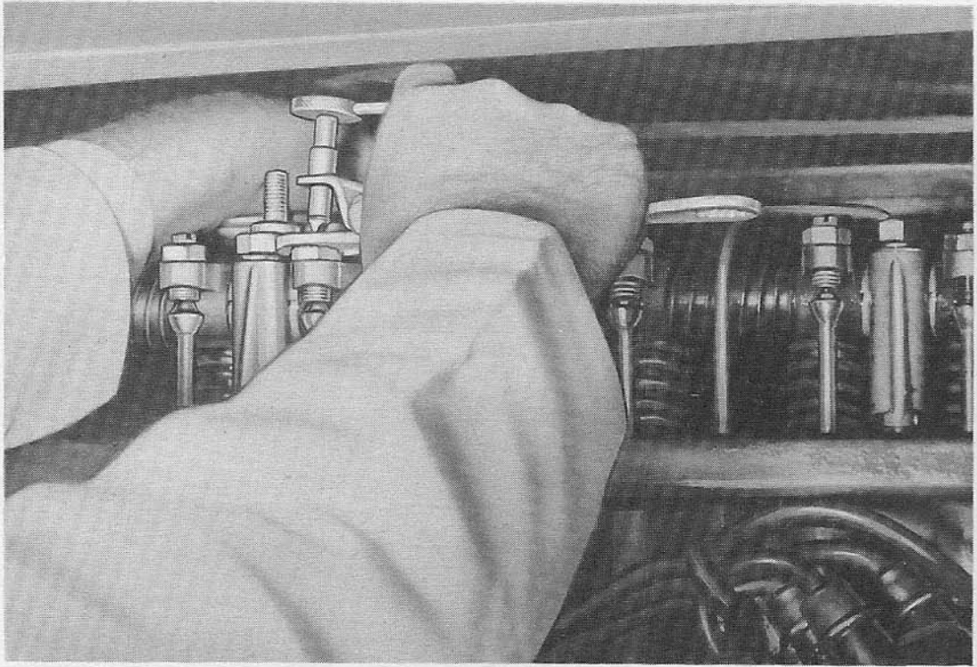
Figure 35 Adjusting Clearance Valve Stem to Rocker Arm
