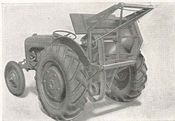
Saw is raised to transport position in one second—ready to move on. Belt automatically loosens on pulleys.
