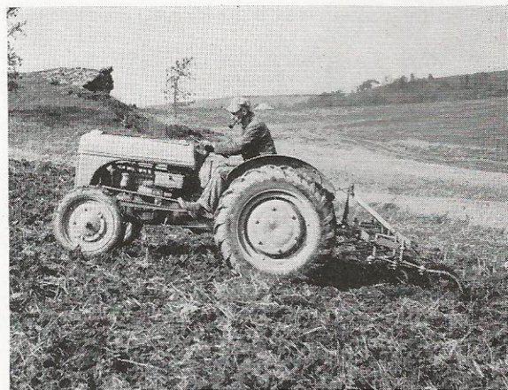
Tines may be changed from row-crop work to general field, orchard or vineyard cultivation, in a short time.
