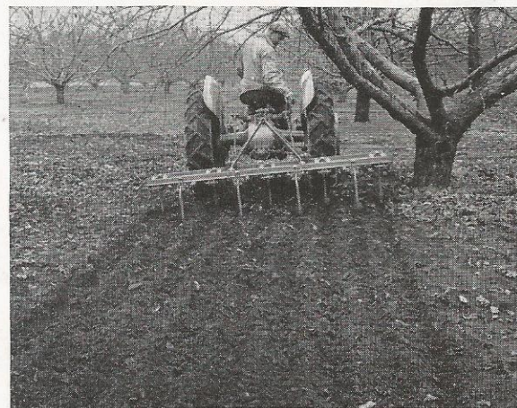
The Ferguson Tiller is made in 5' size for deep subsurface tillage, or for use in heavy soils; and in 7' size for lighter soils and shallower work. Above, cultivating an orchard with 7' Tiller.
