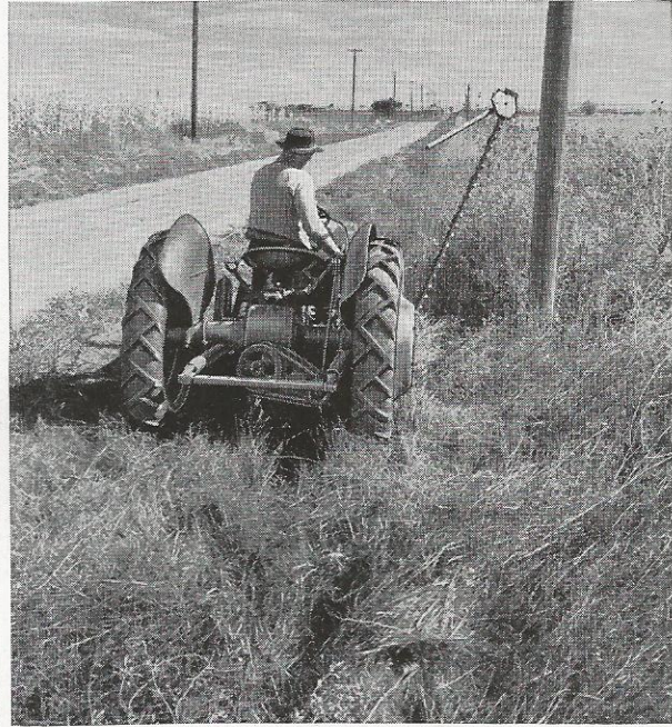
Cutter bar is raised by finger tip hydraulic control.
