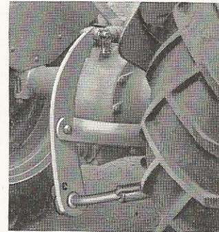
Showing connection to the Ferguson Hydraulic System
