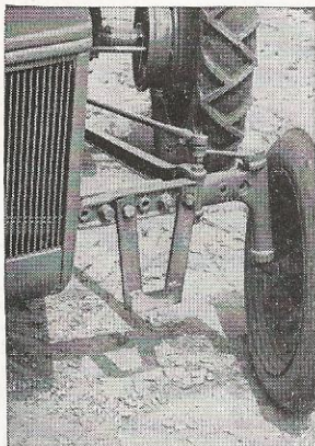
Stirrup bolted to axle Supports I-beam frame
