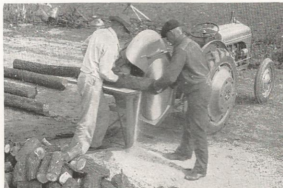
Rests firmly on the ground in working position, anchored to tractor by three-point mounting.
