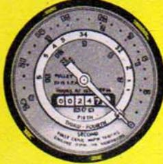
THE "PROOF-METER"-- ANOTHER FORD FIRST-- RECORDS THE HOURS WORKED AND TELLS YOU INSTANTLY THE ENGINE PTO, BELT PULLEY AND GROUND SPEED... FOR TOP PERFORMANCE AND ECONOMY.
