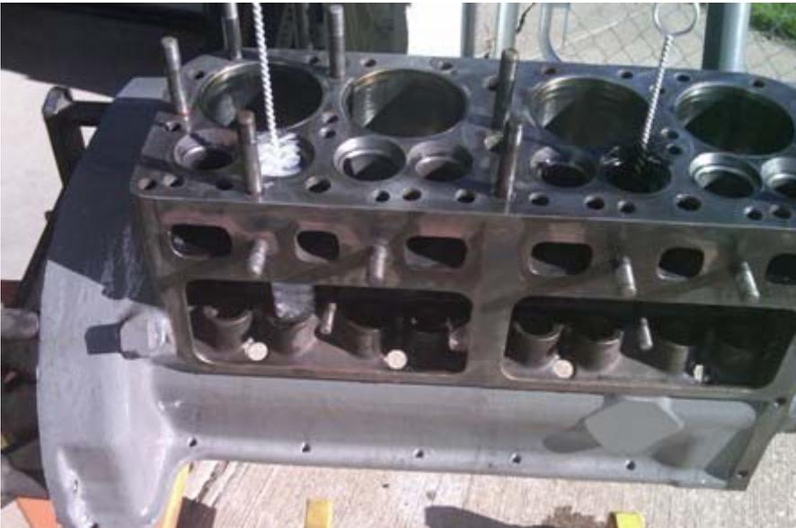
You must also clean the oil galley and 3 passages to the cam journals and 1 passage from the oil pump to the relief valve hole.
