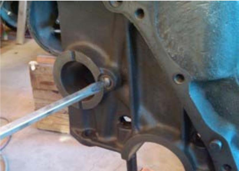
If using adjustable tappets, back the adjusters out and add a couple drops of oil to the threads. These can be very tight and hard to break loose initially; it's easier here than in the block with the Johnson tappet tools. Set the tappets aside. You can place a screwdriver through the tappet to hold it while loosening the adjusting bolt.
