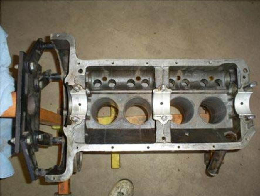
Carefully set the crankshaft in place. Cut a strip of Plastigage (.001-.003) the width of the each main bearing journal and lay on the crankshaft journals. Place the other bearing shells in the main caps and install in place with the arrows pointing towards the front of the block. Torque the bolts/nuts to the correct setting.
