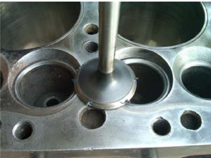
This motor has newly ground seats and the seat face is narrow producing a narrow gray band. On older motors with worn valve seats the band will be wider. Once lapped the valves must be kept mated to their position. I use a center punch and punch dots on the tops of the valves indicating which cylinder they belong to.
