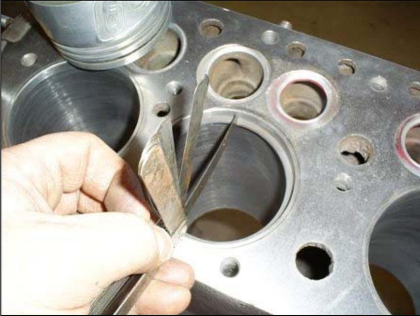
Assemble the pistons. Install the wrist pin keeper in one end, then slip the wrist pin in and the keeper from the other end. Use engine assembly lube on the pin and inside of the rod bushing. There should be virtually no play with the pin in the rod and should only move where intended. Side to slide movement is normal. Ensure that the keepers are seated properly in the pistons. If the keeper comes out the wrist pins will work loose and hammer the cylinder sleeve forcing a rebuild.
