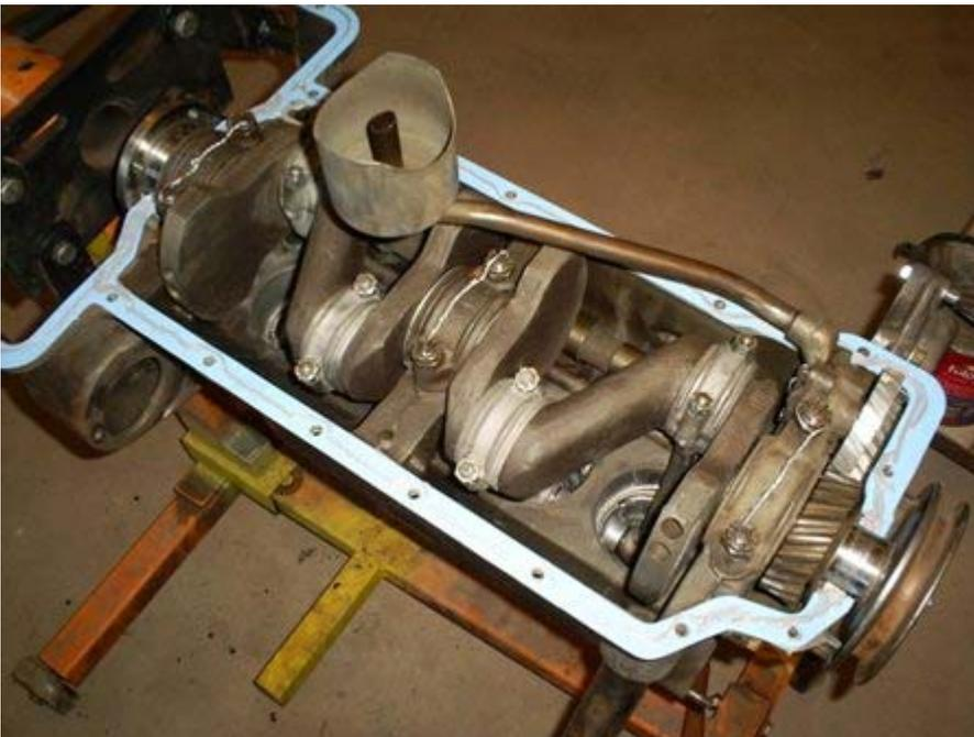
Carefully set the pan in place by landing it in the right place requiring little wiggling. The pan will require a little force to set down as the crankshaft seals are compressed. Start installing all the pan bolts and work from end to end tightening gradually as you go drawing the pan down tight. Do not over tighten the bolts and do not try to tighten them in one move. The pans can be cracked if not installed correctly
