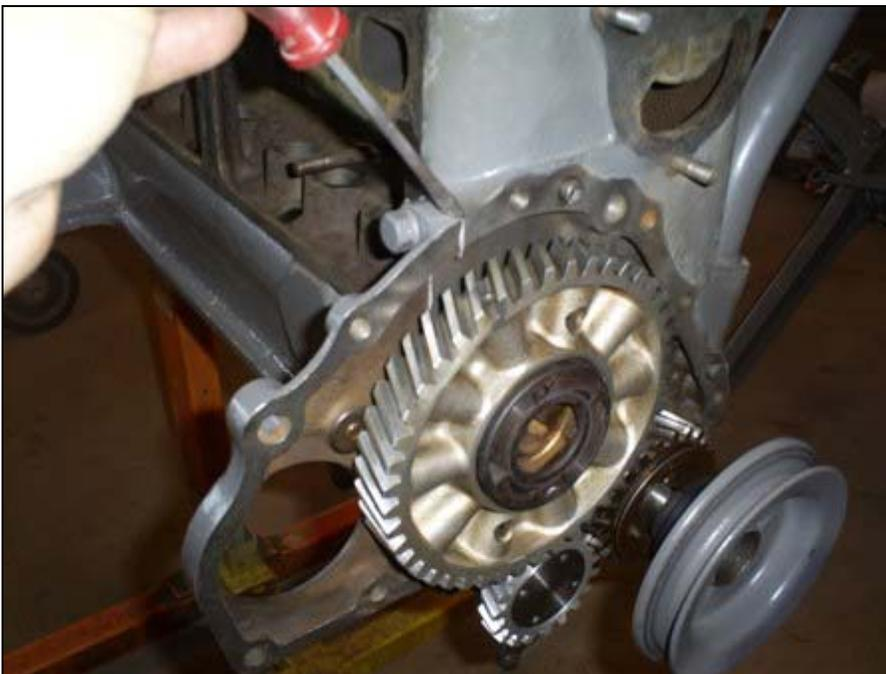
Here the timing cover gasket has been installed using a light coat of Ultra gray silicon. Installing the cover requires 3 hands, once in place it slips over 2 dowel pins and the front neoprene seal and the pulley can then be moved into place. Ensure that the pulley and slinger line up with the woodruff key. I use a marker and place a line on the end of the crankshaft showing where the key is.
