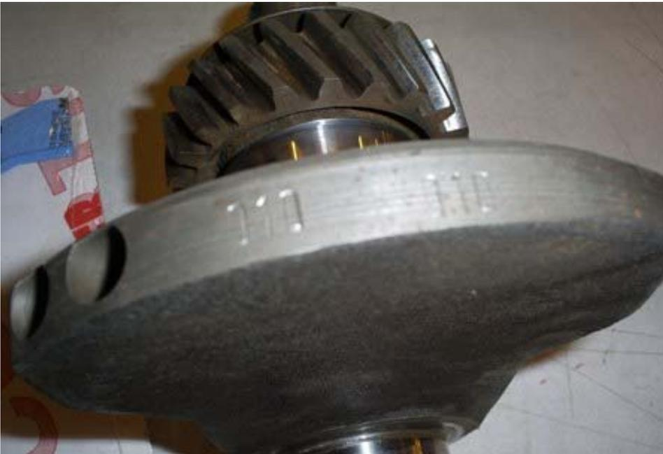
Verify that your bearings match the crankshaft. This bearing shows .010 meaning .010 undersize. It's nice to see it on the box but check the bearing.
