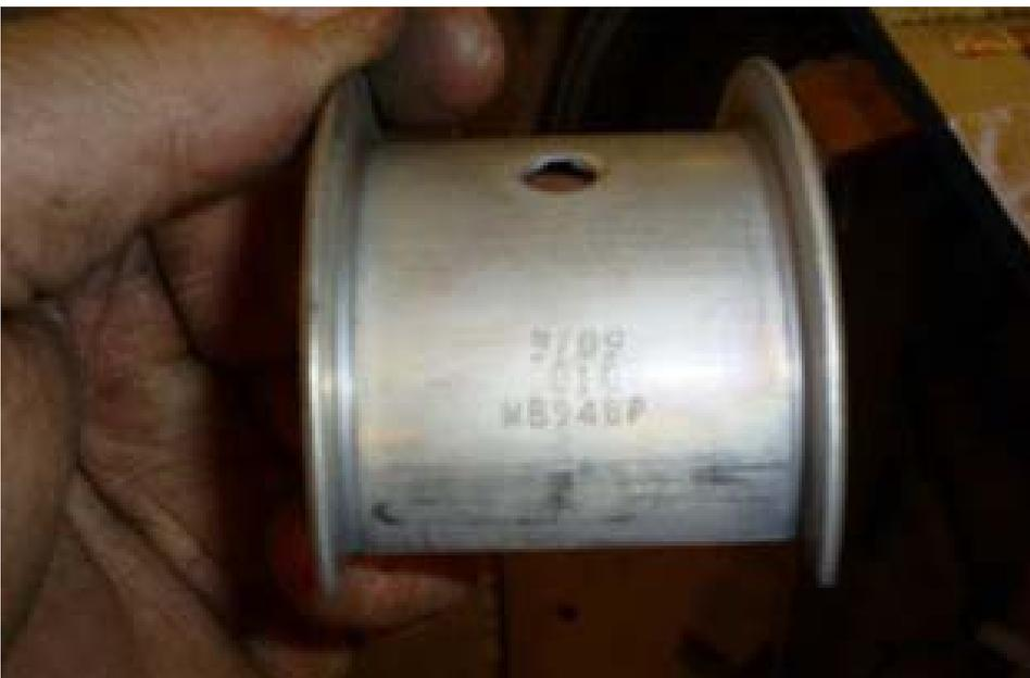
With the engine block securely fastened on a motor stand, place 1 bearing shell in each of the main journals. Notice that the rear seal has not been installed yet. Lightly oil the bearing surfaces.
