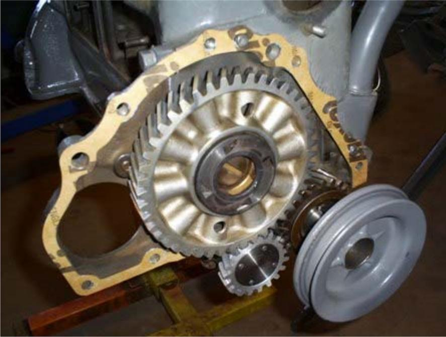
Add some sealant to the groove that holds the front crankshaft seal. With the seal spaced out from the motor, carefully lower the front cover onto the seal then work the cover back onto the motor lining up on the 2 dowel pins. Once located gently work the pulley back towards to motor. Install the crankshaft nut and tighten.
