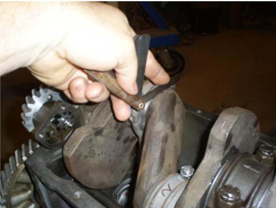
Rotate the crank following the installation of each piston. While new pistons/rings/sleeves will have some drag the crank should still rotate smoothly. On my motor with 2 pistons installed the torque required to turn the crank was around 20 ft/lbs.
