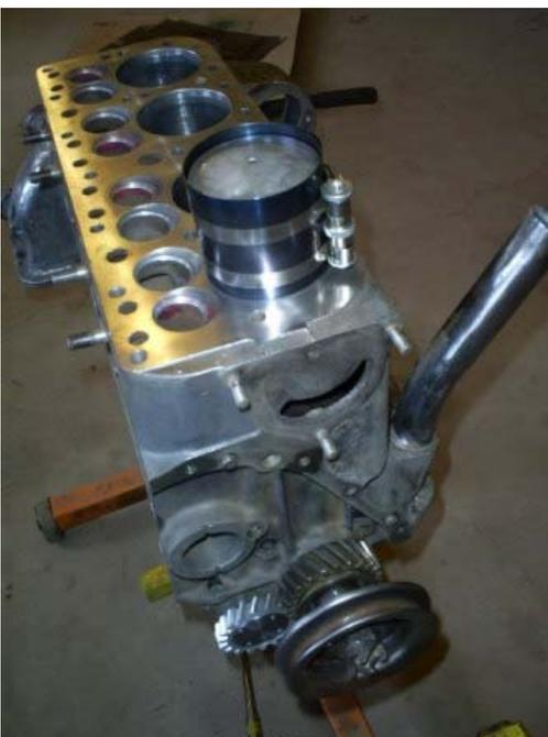
With the connecting rod in, place a strip of Pastigague on the crankpin and install the bearing shell and cap and torque to specification. Remove the cap and confirm that the rod bearing clearance is correct. This is the only reliable way to know that the clearances are correct. Once happy, clean the Pastigague off, lube the other bearing shell and install the cap. Repeat the process for the remaining pistons
