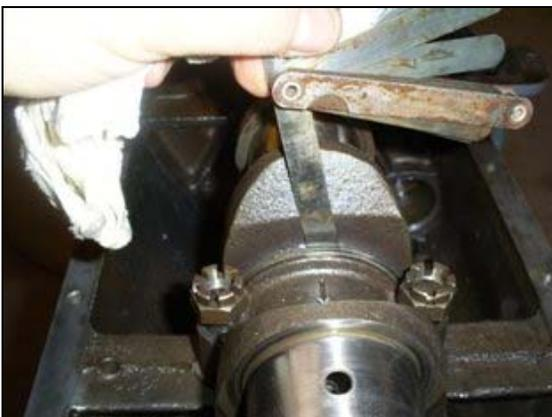
Once the crank is in slip the front pulley and nut on and see that the crank will turn. It may be tight initially but will loosen up. Make sure the rear seal ends do not get lube on them. On my motor, the crank with the main bearings installed and top half of the rear rope seal required around 10 ft/lbs to torque to rotate. The initial rotate is a little higher and quickly lessens as the crank is spun. It should rotate freely with no tight spots or binding.
