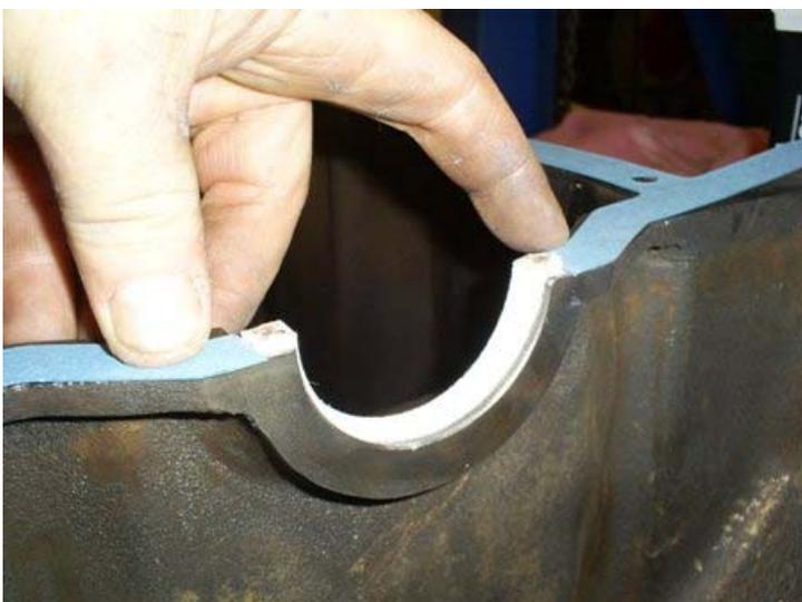
Prepare the front seal on the pan. Place the 1 piece neoprene seal in its groove and cut the pan gasket so that it butts up against the seal.
