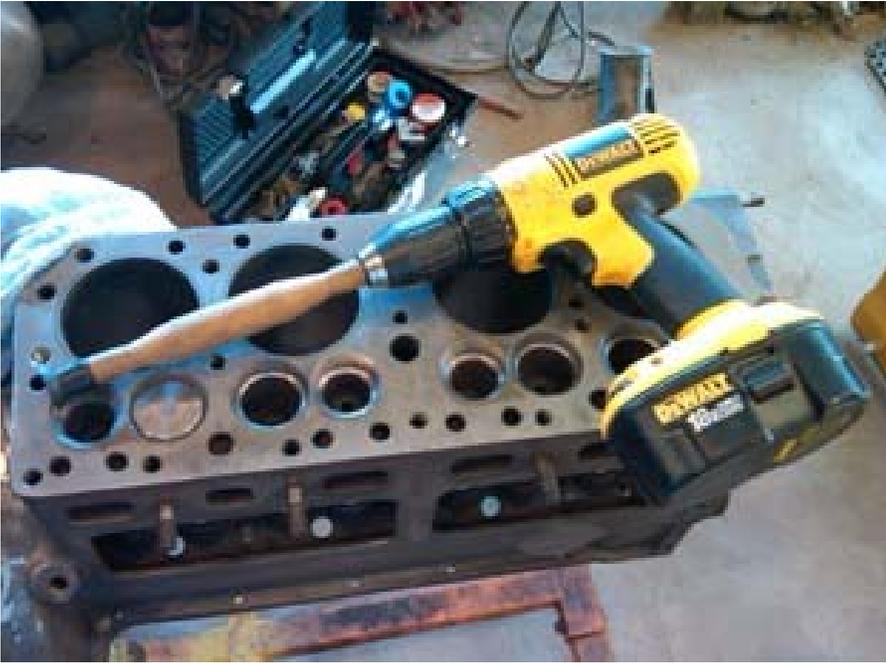
The valve seats are hardened and lapping by hand is very time consuming. I use a variable speed drill running moderately slow guided by my hand with a small amount of lapping compound. Valves are lapped until there is a continuous gray band around the valve.
