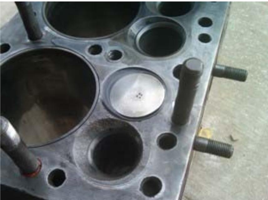
This particular block is one where the valve seats were not ground, just lapped. The valve seat faces are wider from use and after lapping have a continuous gray color band which is also present on the valves. There should be no pitting in the valve seats or they should be ground.
