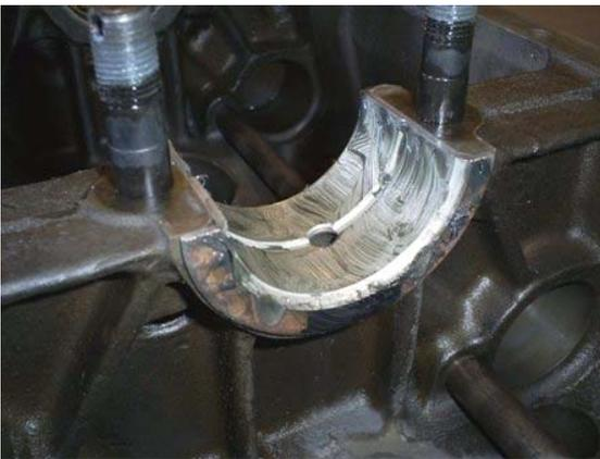
Gradually torque the bolts/nuts to the proper setting while rotating on occasion, the crank should not bind up as the caps are tightened. The crank should be lightly tapped towards the rear and the end play checked at the center bearing.
