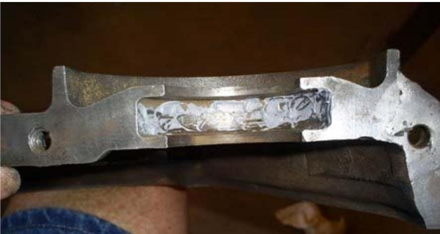
Once on your motor should look like this. Use a temporary bolt for the lower governor bolt hole to hold the parts in place as the sealant dries. Gradually tighten up all bolts that contain the timing cover and governor mounting plate.
