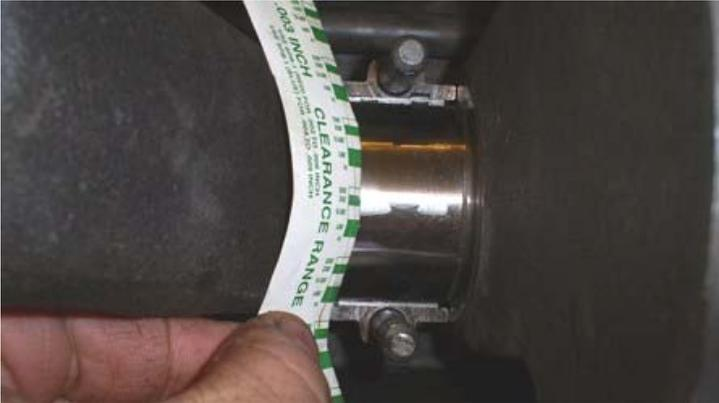
As each piston is installed, check the rod side clearance the same way you checked the crankshaft end play. Gently tap each rod to 1 side then check the clearance between the cap and crankshaft.
