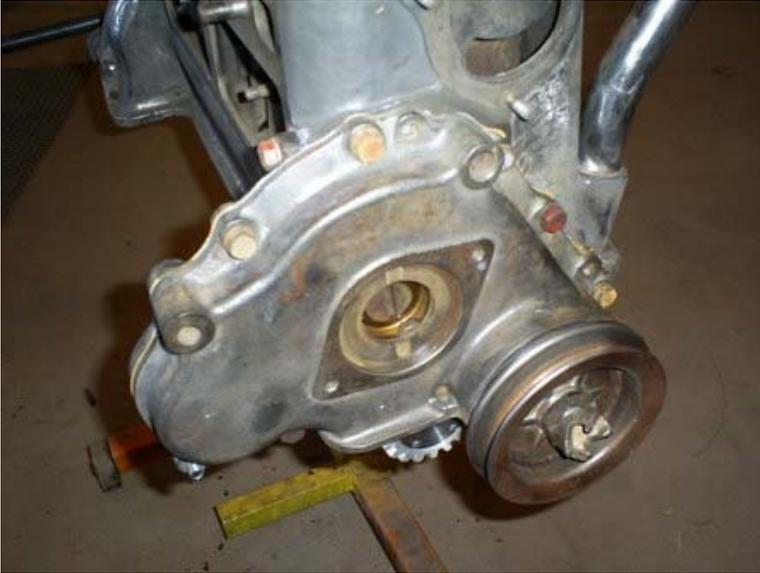
Oil Pan installation. The rear seal was installed earlier. For the rear seal we are not overlapping the seal with the pan gasket so the rope seal is cut flush to slightly higher than the block, and slightly taller than the pan and gasket creating a slight interference. Lube the face of the rear seal with assembly lube keeping the ends clean.
