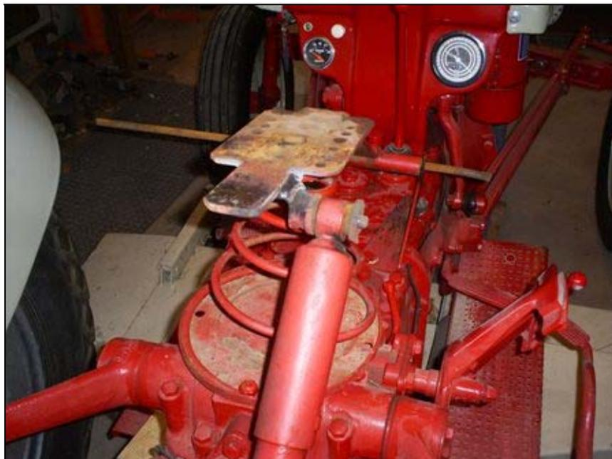
The Shock was test fitted with its new location and everything checked out ok.
