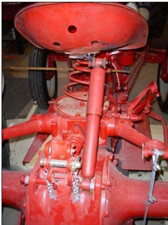
All the parts were cleaned and painted, A new shock was ordered from Steiner Tractor Parts. Here the finished seat has been assembled and installed on the tractor.
