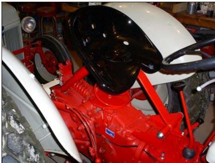
In this view you can see the notch I made in the spring mounting plate to allow for shock compression. I also removed the position control lever which is bent from the factory and straitened it. This eliminated the interference with the spring mounting plate.
