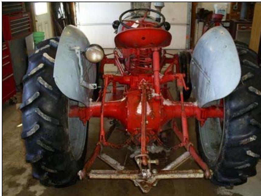
Since I mow frequently with an 8N I decided to make this seat fit an 8N. The first step was to set it on the 8n and see if it was even possible. The rear shock mount was not, due to the differences in the rear center housing the existing bracket could not be used. The coil spring mount on top of the hydraulic cover interfered with the position control lever.
