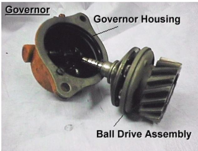
When the thrust measurement is right, reinstall the ball drive shaft into the Governor housing. Hold the bearing base against the housing and ensure that the shaft spins freely without binding or grinding noises.
