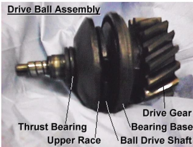
From left to right, Ball Drive Shaft Proofmeter drive end, retaining clip, washer, shims, fork base, thrust ball bearings, upper race, steel balls, ball retainer, lower race, bearing base, fiber spacer, and drive gear.
