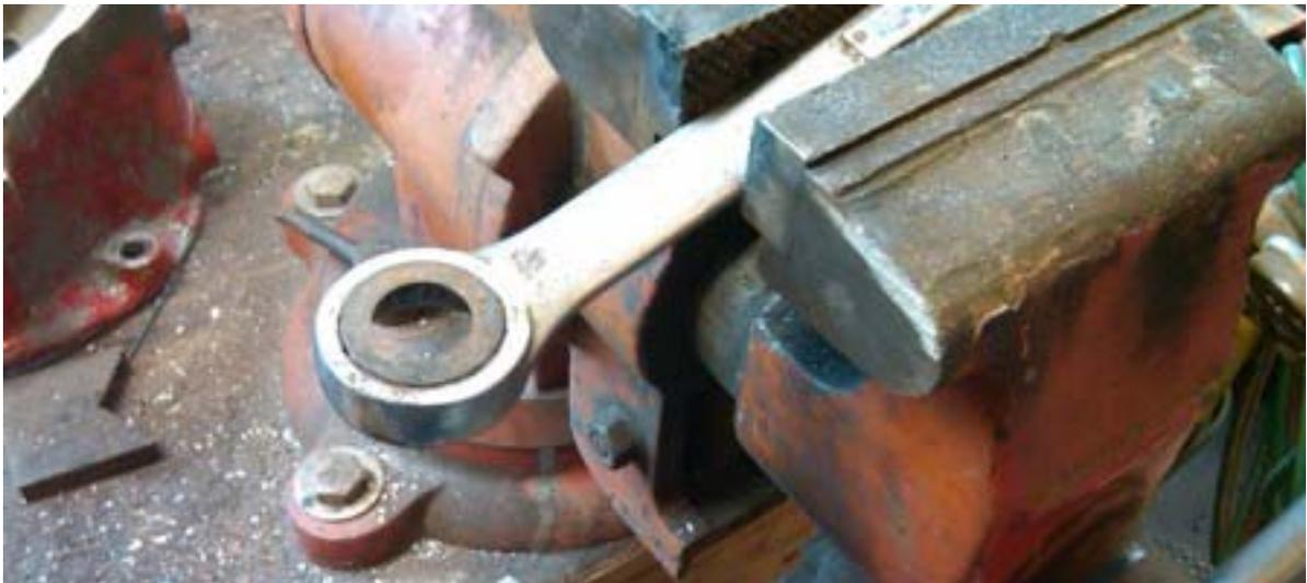
I changed over to a 1.0625 wrench and did the same step again, this time the shim fit the bottom of the shifter ball like a glove. Here's a picture of the new shim prior to being brazed to the shifter lever. In this picture you can really see how much lower the lever is and keep in mind when moving the lever to the right the slot would have to be lower yet. I could have simply cut the slot lower but I wanted to try to fix this one as my shifter drags on the transmission gears in neutral.
