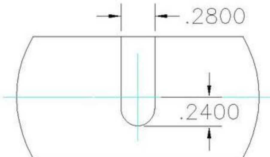
The slot was cut by locating the center for the bottom radius and drilling a hole of the proper size. The sides were cut with a Dremel moto-tool with small abrasive cutoff wheels.
