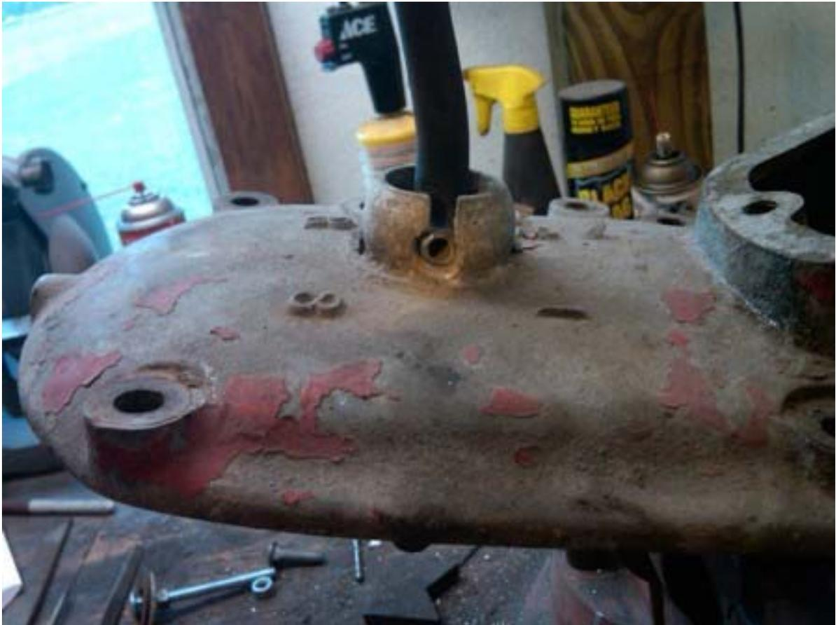
I sent my cover to the weld shop and simply asked that the worn slot be welded shut. It came back welded up and roughly shaped. The part required additional working with die grinders and a Dremel tool. Once I had the shape dialed in it was time to cut the slot.
