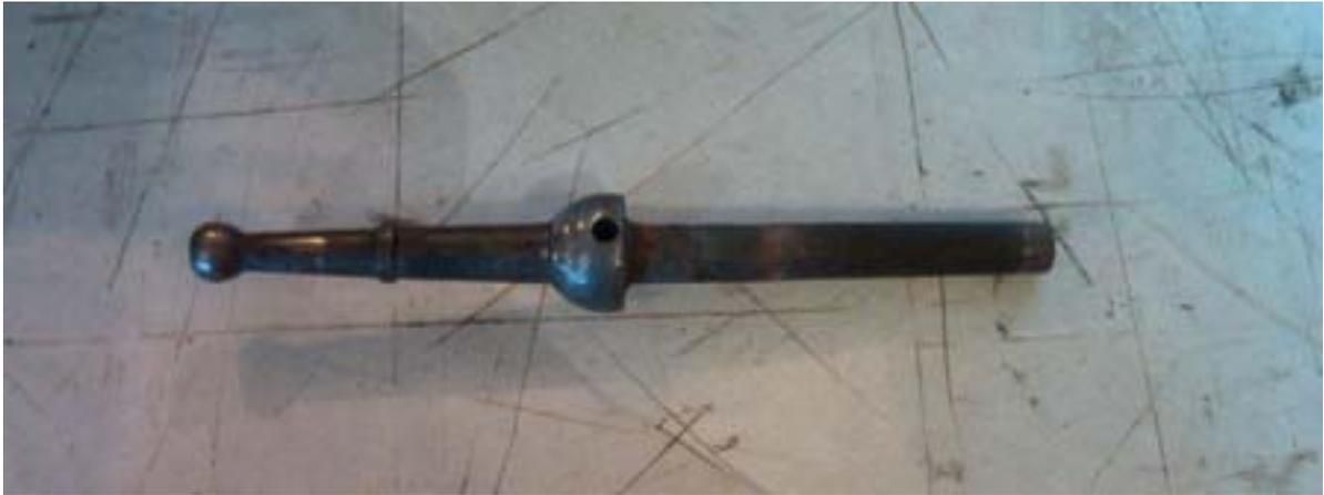
The wrench was placed in the vice; the bearing was set on the wrench. I heated the bearing bright red then punched it with my die. The first set was close, but it didn't fit the lever tight enough yet and didn't fit well in the wrench any more.
